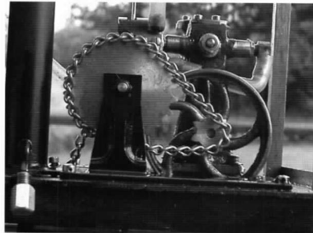
**Above:** Cast engine-drive side. I dressed up the jack shaft supports. Note gate for reversing valve and cap of condensate tank drain.
