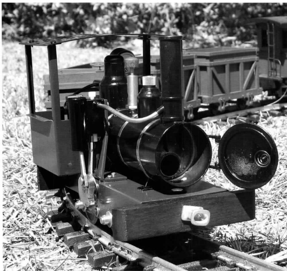
*With the smokebox door open you can see that the author has removed the exhaust condensate tube for easier lighting and better reliability of the burner (see text for details). The manufacturer has implemented this and other changes on all current production.*
