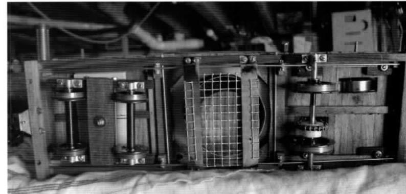
Underside of bar stock engine logging loco. Note truss rod detail, boiler support, drive axle, cut out in floor for flywheel.
