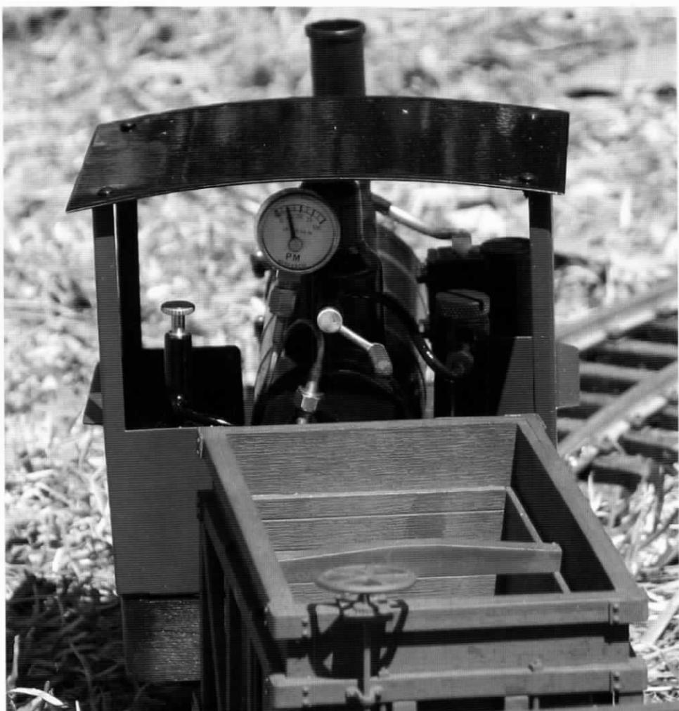
*A peek into the cab from the rear. From left: gas control valve, pressure gauge, throttle and displacement lubricator.*
