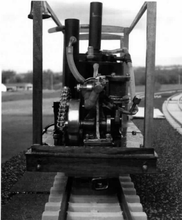
**Above:** Front view of cast engine logger. Note safety valve on boiler above the engine. Pocket coupler is used when double heading with the other logger.
