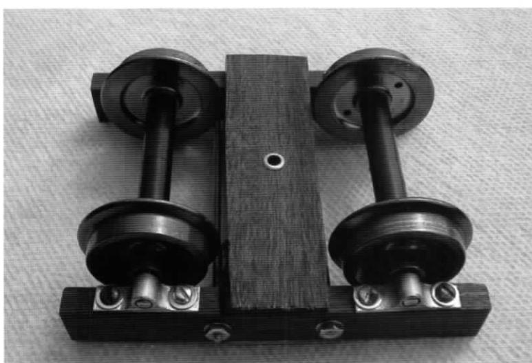
Truck with Bachmann small wheel sets. Note: homemade axle boxes, pivot bushing. Nuts are for rods holding the wood in compression.
