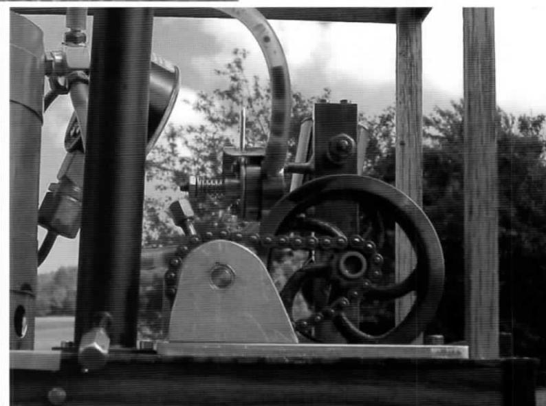
Bar stock engine. Drive side. Chain pitch is .1475". Chain and sprockets are pricey but neat.
