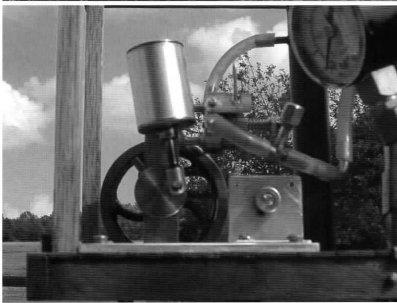
Bar stock engine. 5/8" bore, heavier flywheel. Pulled 32 axles.
