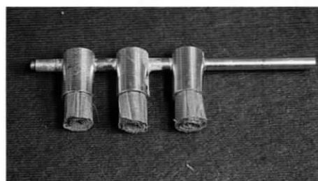
The wicks should be trimmed to the proper height above the top of the burner cup. This height will vary for each application.
