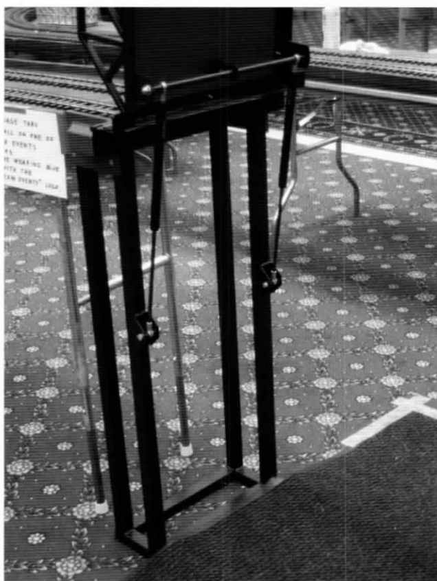
With the bridge in the open position, the mechanism is visible.
