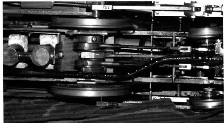
Typical valve gear and burner arrangement.
