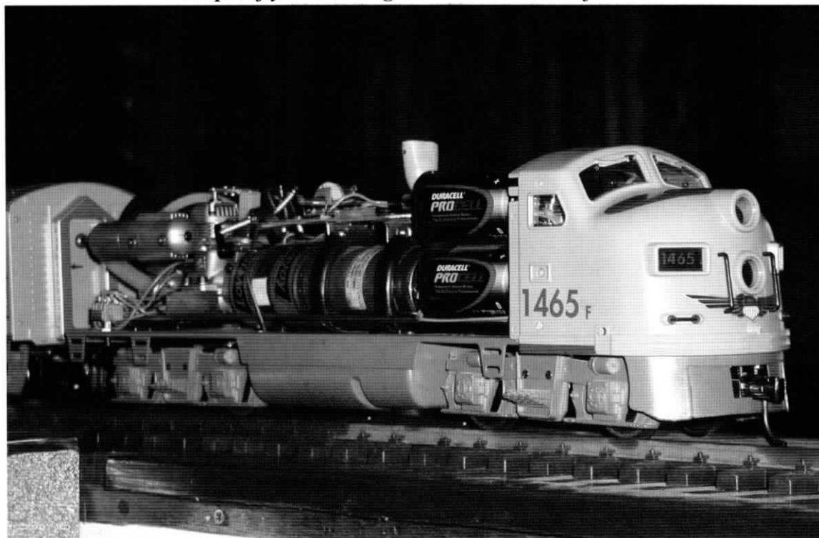
Above and below: The F7 with the hood removed. Note the engine, coupler/flywheel and generator on the sub-frame.
