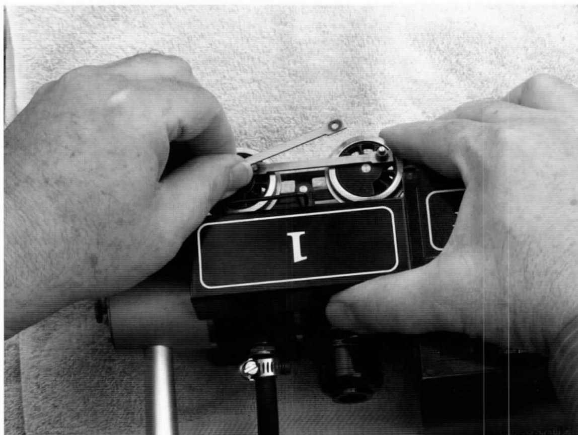
Disconnecting the big end of the main rod from the crankpin (see text).
