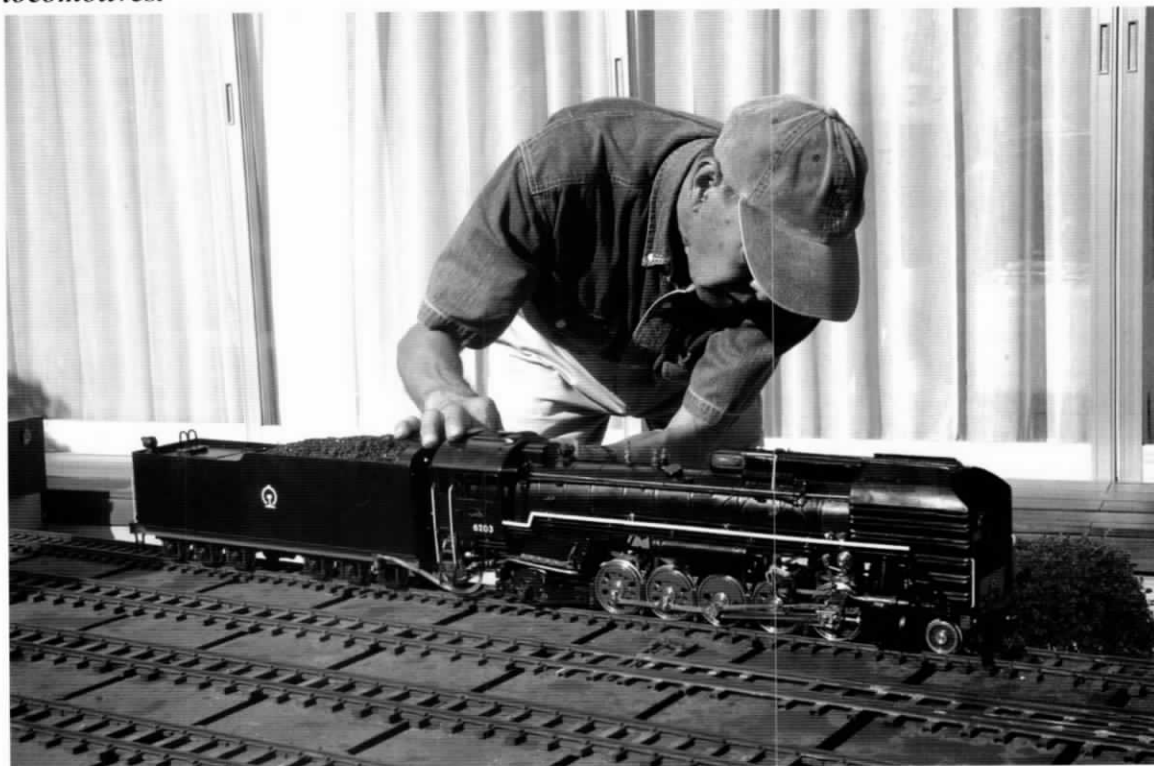
Master builder Mr. Kazuo Yano with his beautiful scratch built, alcohol fired Chinese Railroad class QJ 2-10-2, modeled in 1:30 scale.
