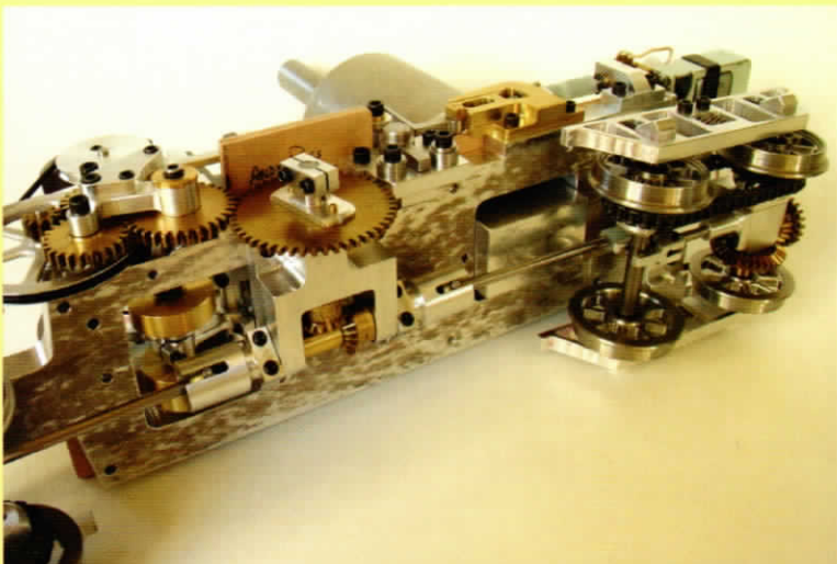
Under the frame are the miter gears, universal joints, and drive shafts transmitting power to the trucks. The frame cut-outs provide clearance for the engine, and air for the burner, respectively.
