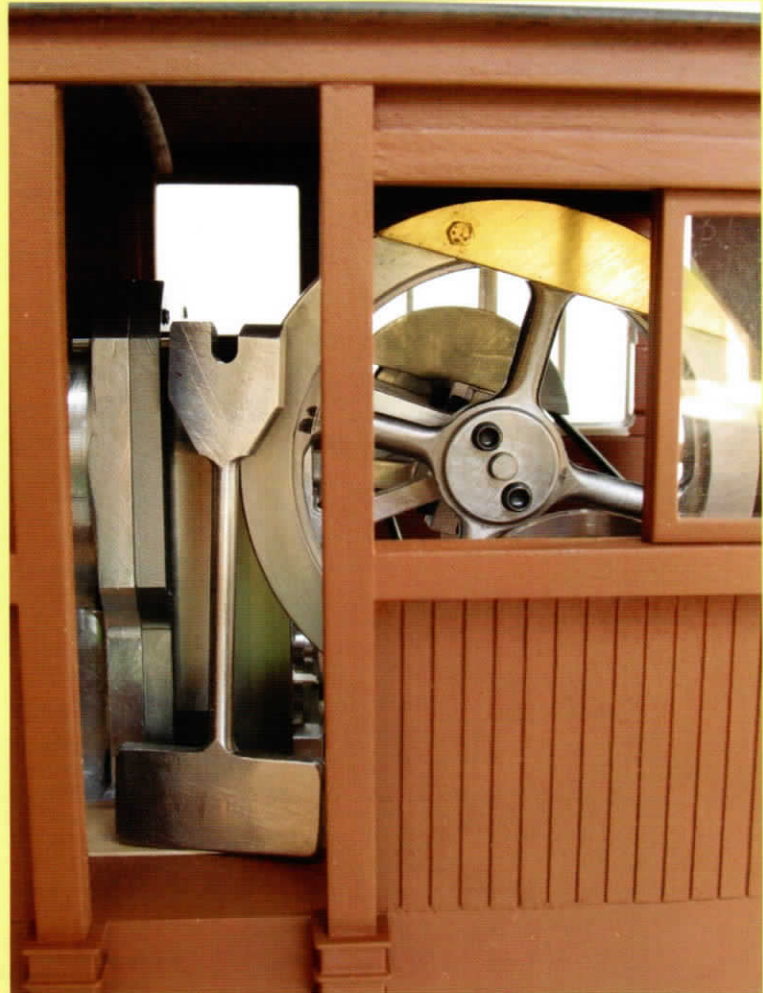
The starting key, standing in the doorway; in use it would poke through the open window and engage the flywheel mounting screws.
