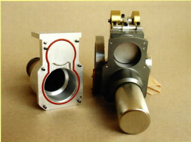
The Stirling engine from the heat exchanger side of the block, with the cylinder head removed. All static seals are O-rings.
