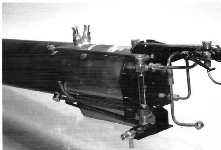
Boiler (item I) - On top of the boiler are the safeties, on the bottom is the blowdown valve and on the body at the backhead is the water gauge and throttle.
