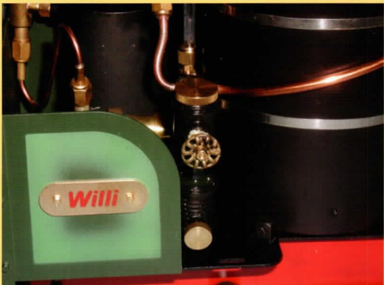
*The displacement lubricator, with knurled filler cap, oil flow control valve and drain screw.*
