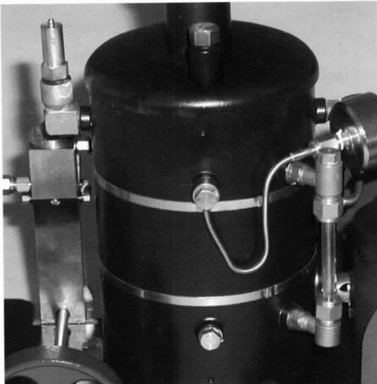
*Willi's boiler. At upper left is the safety valve. The bush on top is the cold water filler, and at the bottom is the bush for the optional Goodall-type valve. The gauge glass (right) is easy to read and very accurate.*
