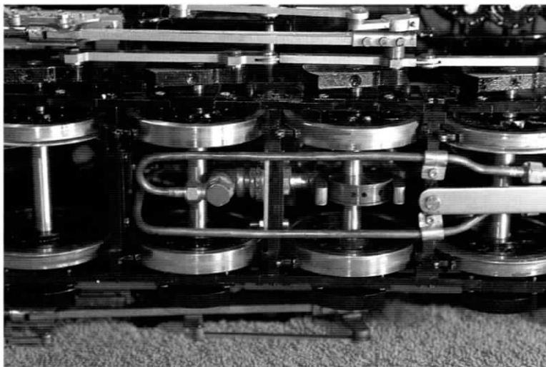
Underside view, showing axle driven water pump.
