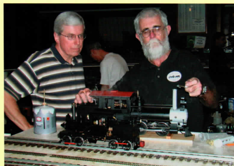
Bill Ford was showing his WLDS (Water Level Detection System), which eliminates the need for a sight glass.
