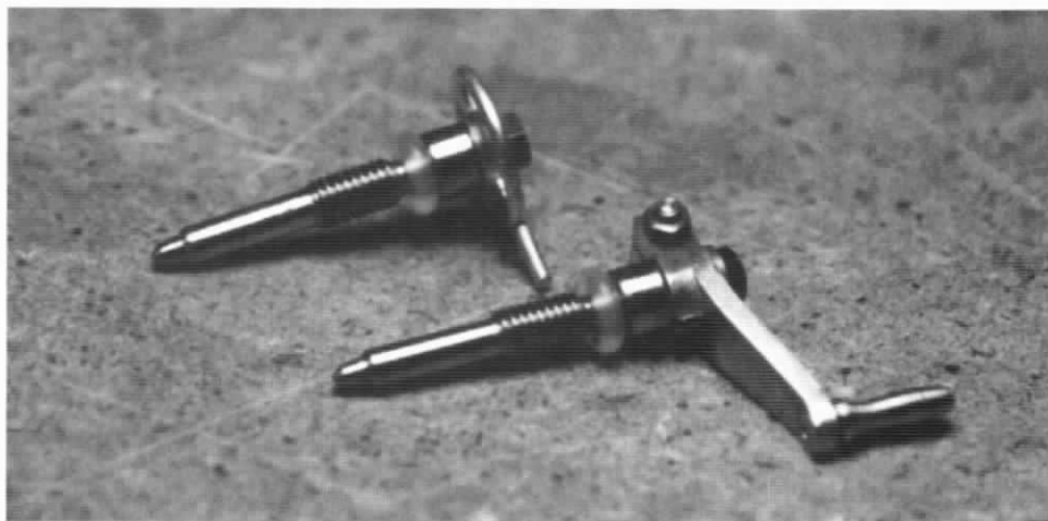
Picture #5 - blower valve and throttle valve modifications.
