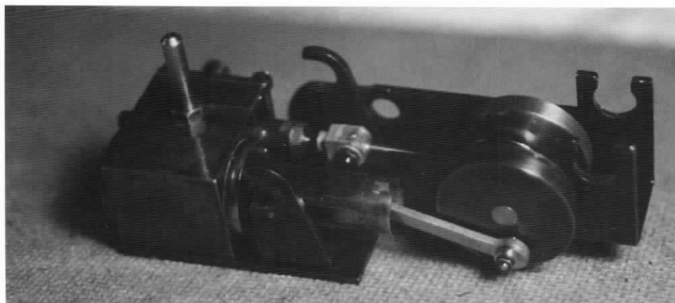
Picture #1 - Aster Lion engine unit, as modified by the author. (See text for details)
