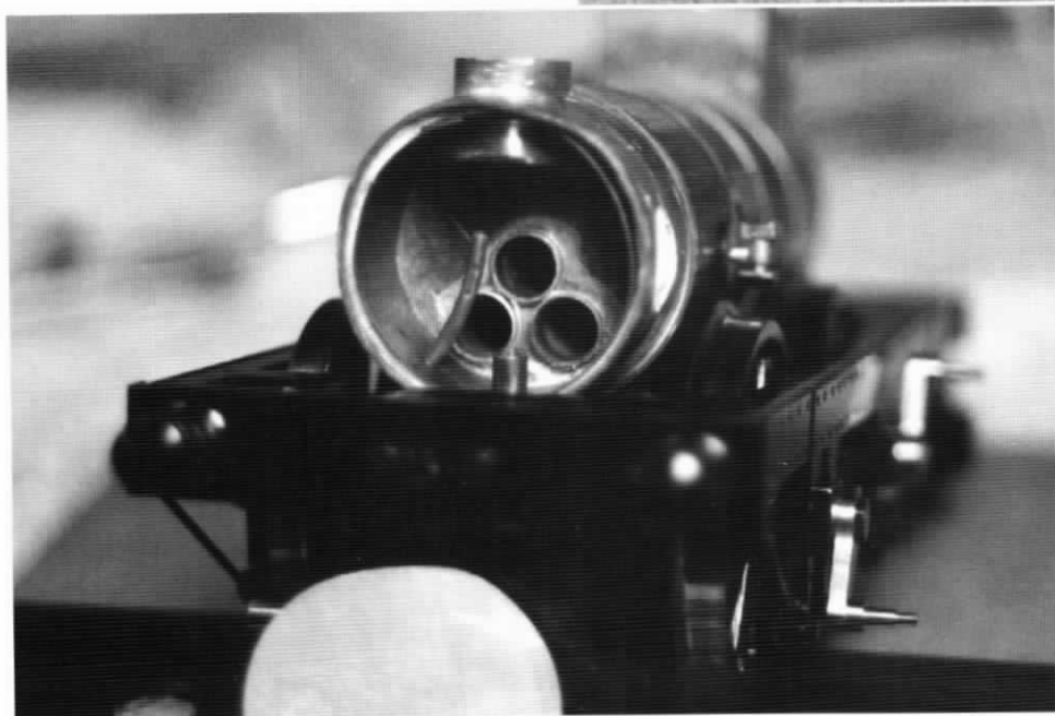
Picture #3 - the author's smokebox sealing modifications.
