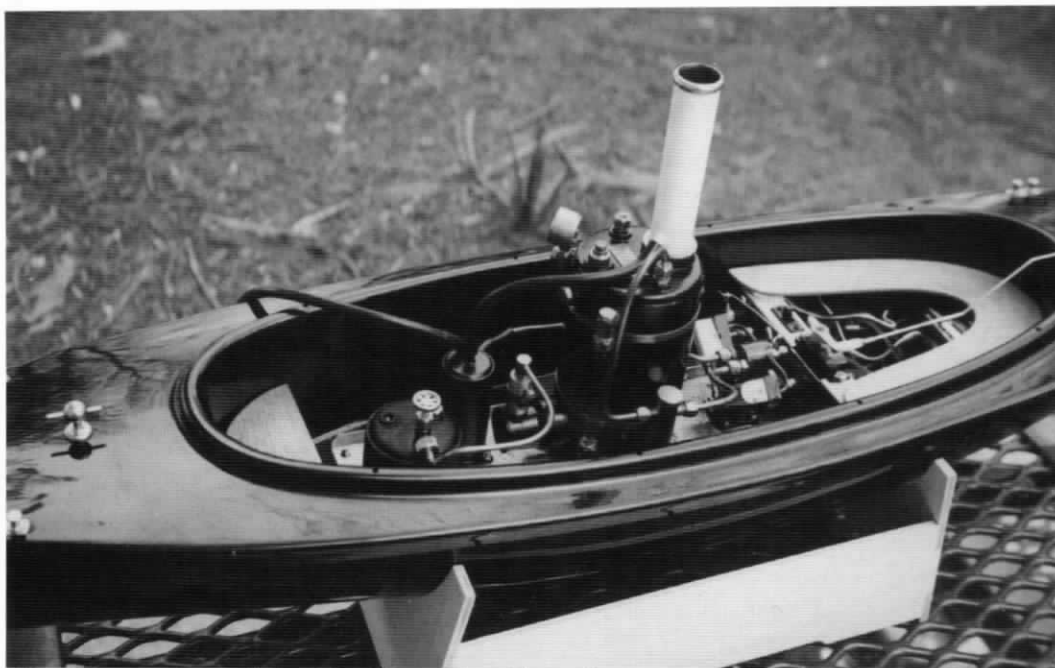
The installation of the Cheddar Pintail marine steam plant in CLAIRE's hull is clean and neat.
