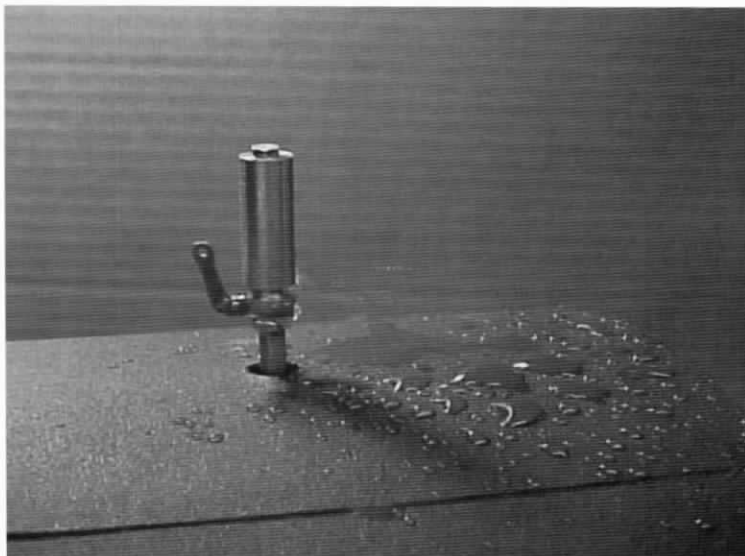
Note the spray and condensation from the safety valve, which the author piped through his decorative whistle.
