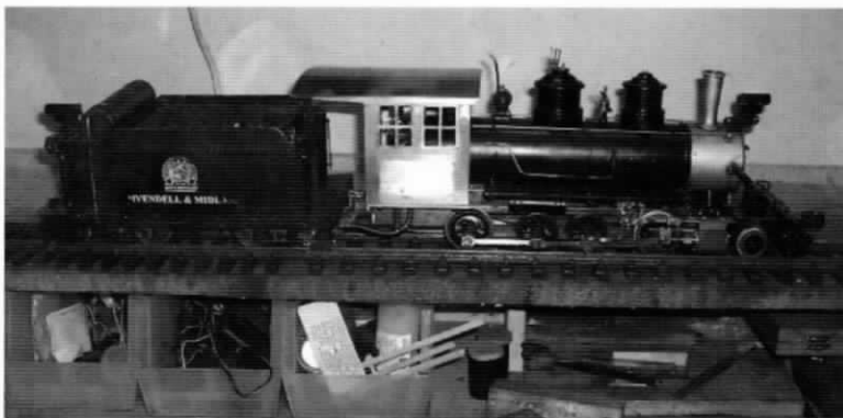
The complete (but unpainted) cab has been fitted to the chassis.
