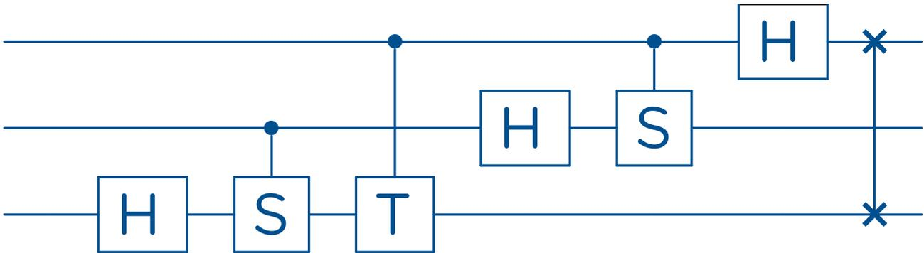
Figure 2: A subroutine of a quantum Fourier transform algorithm, to be read from left to right. Each row is a single qubit. Squares with H represent a single-qubit rotations called Hadamard. Vertical lines represent two-qubit gates.
