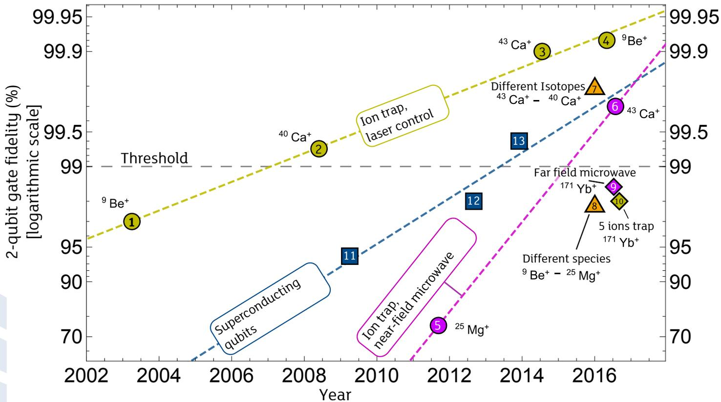
Figure 3: Progress of ion-qubit and superconducting qubit technology over time. y-axis: 2-qubit gate-fidelity (precision), in logarithmic scale. Above the threshold of 99% it is possible to reduce errors using the surface code error-correcting scheme.
