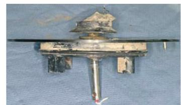
Bent vane shaft, still in place in the upper bearing on the top of the sensor
