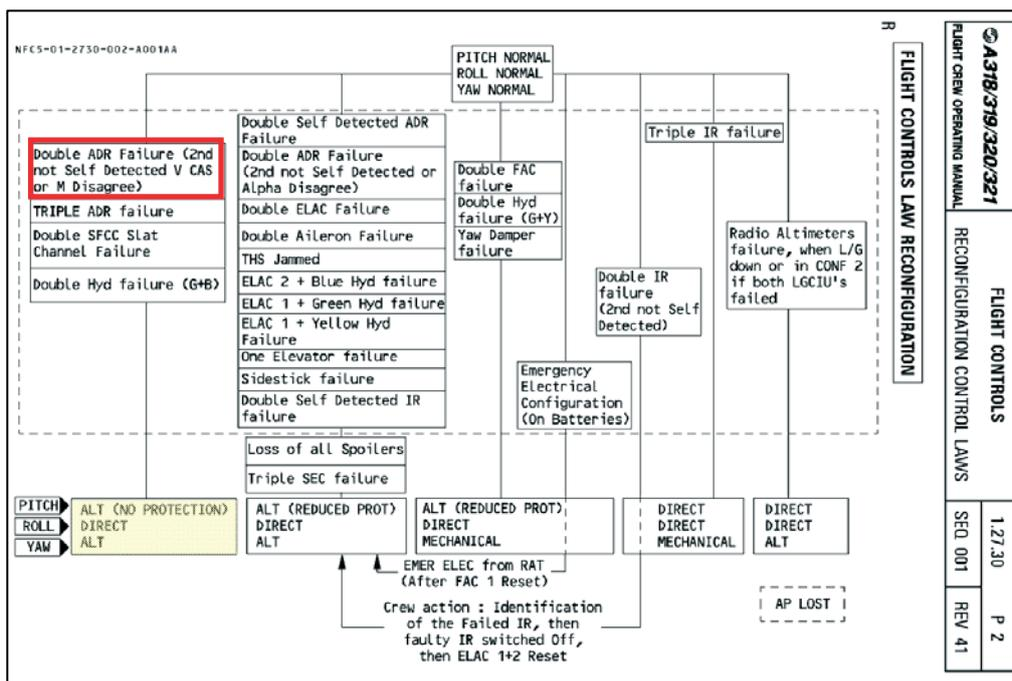
At 15 h 45 min 40 s, the pitch flight control law passed from direct to alternate. The recorded pitch angle was then above 50 degrees, which indicates a change to unusual attitudes law (phase 1). The load factor then not being between 0.9 and 1.2 g over a sufficiently long period, phase 2 of this law was not subsequently triggered.
