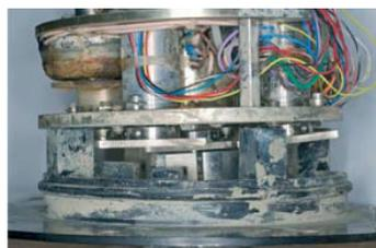
Solenoid and two resolvers with pinions out of line
