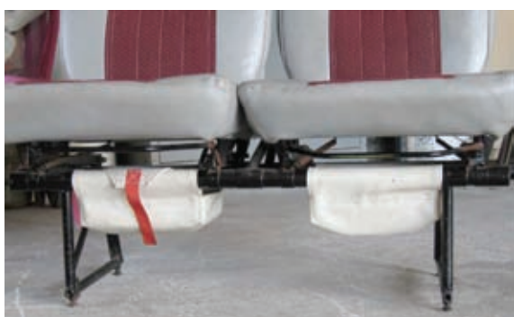
Figure 10: removed seats and stowage pouch with an accessible red pulling strap (left) and with an inaccessible pulling strap (right)
