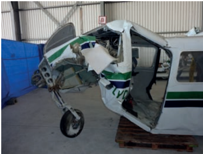
Figures 5 and 6: side view of the deformation of the aircraft nose and cockpit (seats removed) Left: damage to aircraft nose, cockpit floor twisted upwards. Right: instrument panel against the roof.
