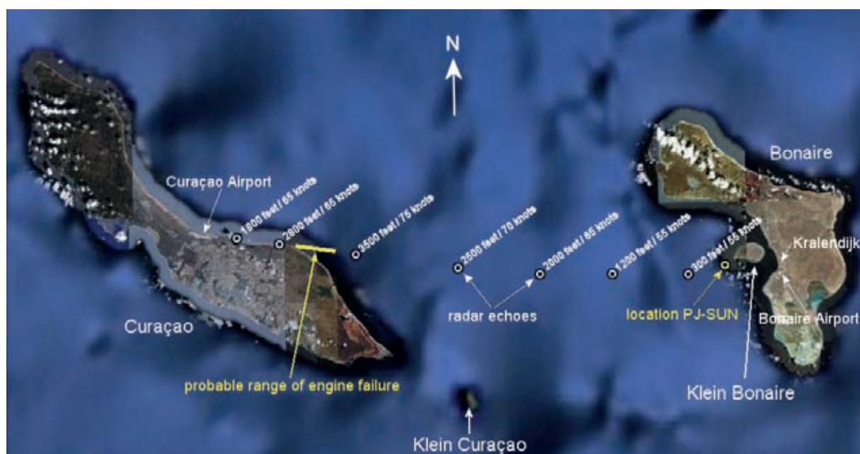
Figure 1: reconstruction of flight DVR014; radar echoes of the aircraft including altitude and groundspeed [sources: Coastguard NA&A and NAATC data]
