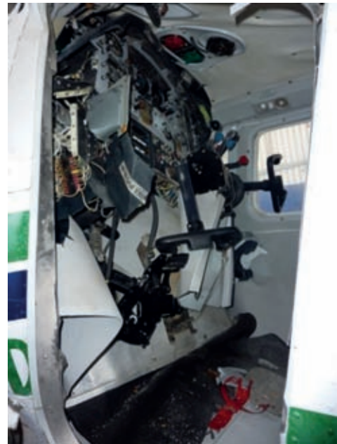
Figures 5 and 6: side view of the deformation of the aircraft nose and cockpit (seats removed) Left: damage to aircraft nose, cockpit floor twisted upwards. Right: instrument panel against the roof.
