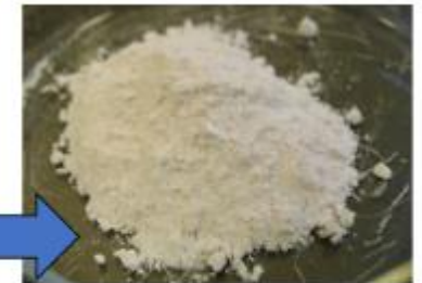
Filtered and dried double salt (further converted to hydroxide, then oxide)
