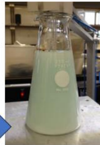
Precipitation by \text{Na}_2\text{SO}_4 addition
