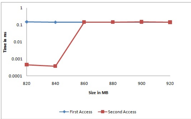
Figure 6. Third run where the step size is reduced to 20MB and starting with 820 MB as the assumed buffer cache size
