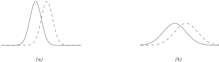
Figure 3.1: Changing the mean of a Gaussian by a fixed amount (from solid to dotted curve) can have more impact when the (shared) variance is small (as in a) compared to when the variance is large (as in b). Hence the impact (in terms of prediction accuracy) of a change to \mu depends on where the optimizer is in (\mu, \sigma) space. From Figure 3 of [Hon+10], reproduced from [Val00]. Used with kind permission of Antti Honkela.
