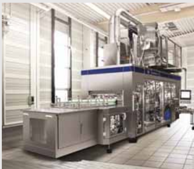
SIG high-performance filling machine CFA 1224-36 with Drinksplus option
