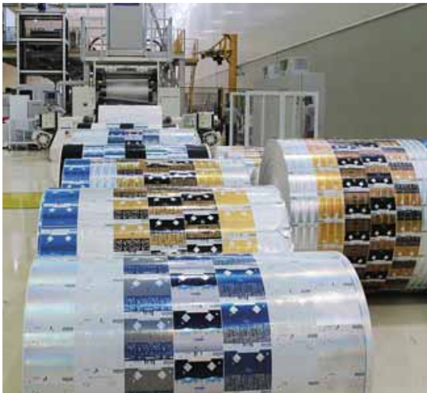
The 6-layer structure is assembled on a Davis Standard extrusion laminator in one go at Asepto, Sanand. Photo IFB
