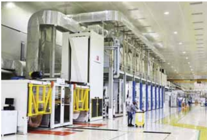
Heidelberg Gallus 7-color Intro 1320 mm wide unit to unit flexo press capable of running at 500 meters a minute and equipped with a Martin Automatic unwinder, autosplicer and rewinder in the Asepto Sanand plant. Photo IFB
