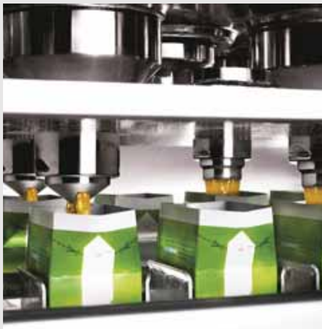
SIG high-performance filling machine CFA 1224-36 with Drinksplus option suitable for aseptically filling CombiblocXSlim in up to nine different volumes ranging from 80 to 200 ml.
