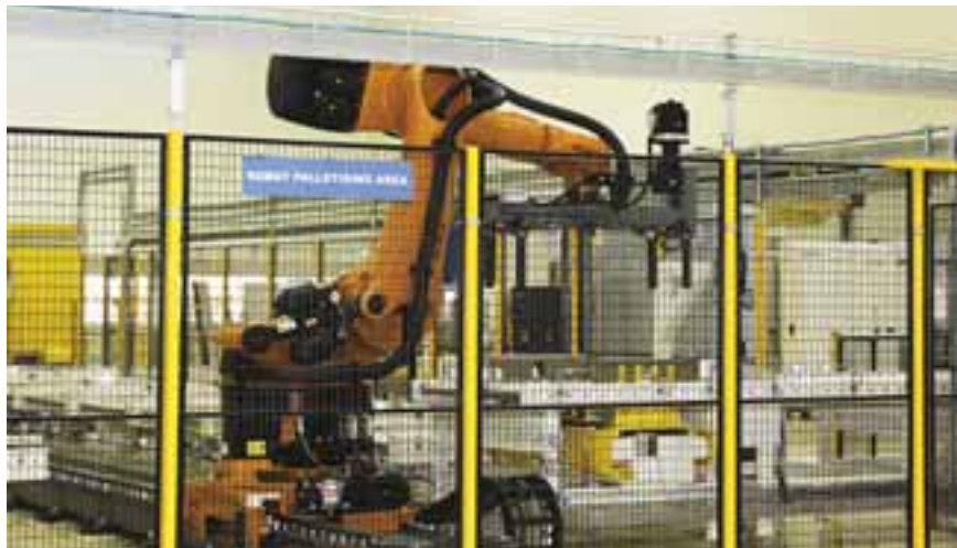
The standard slit reels of laminate are stacked on pallets and wrapped by an automated robotic logistics system from ITW Signode with 16 stations helping to maintain the end-to-end hygiene of the process. Photo IFB
