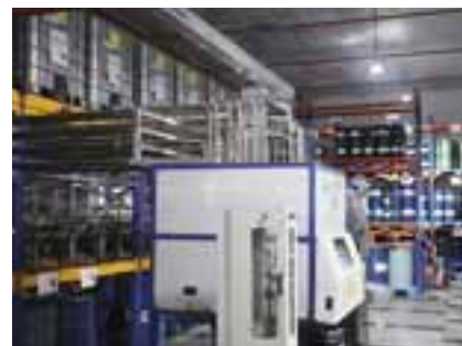
Parakh Flexipacks has an in-house automated ink formulation and mixing plant from Siegwark for its entire CI flexo printing needs. Photo IFB
