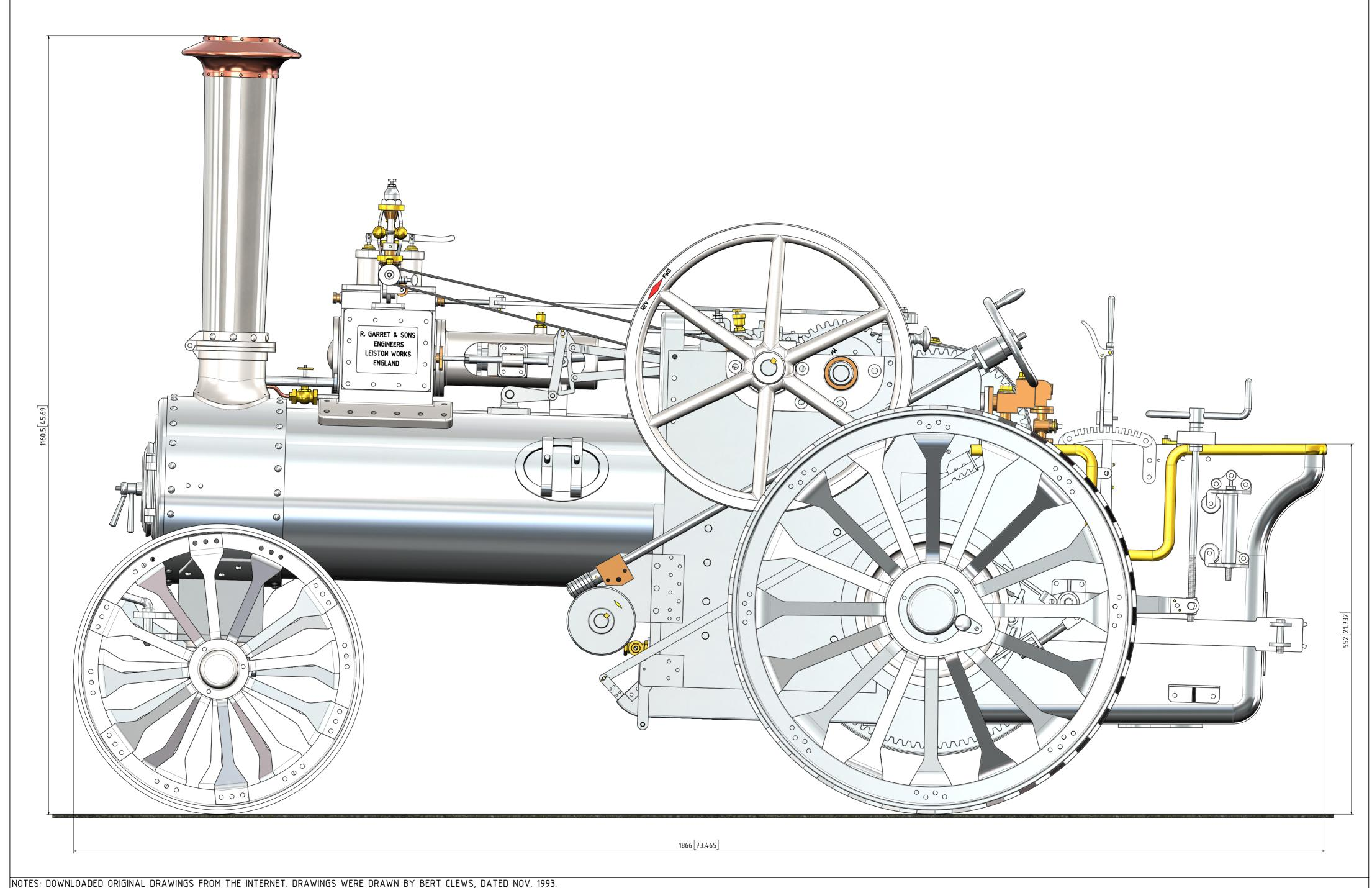
A MODEL OF A "GARRETT" TRACTION ENGINE GENERAL ARRANGEMENT
