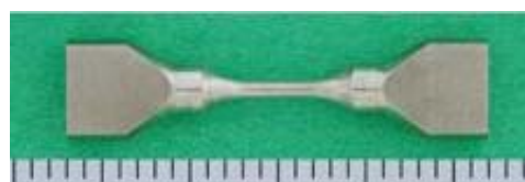
Fig.1 Specimen shape of low-cycle fatigue tests (mm)
