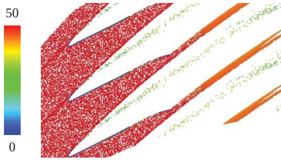
Fig. 5 Droplet Distribution and Speed [m/s]
