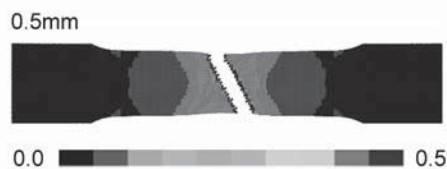
Fig. 5 Contour plots of the equivalent plastic strain distribution after fracture by SPG
