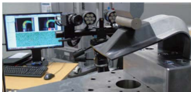
Fig. 17 Test setup for fiber-reinforced PA6 plastic parts
