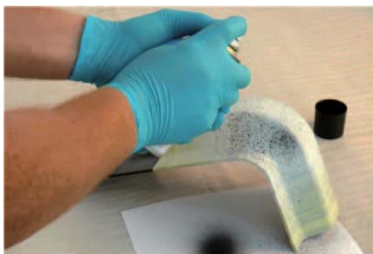
Fig. 10 Surface preparation with a stochastic pattern
