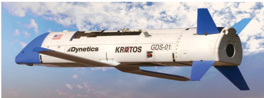
◀ A Dynetics-built X-61A Gremlin flew over Utah under a DARPA-sponsored program to test the feasibility of launching and recovering cruise-missile-sized drones from conventionally piloted aircraft.
