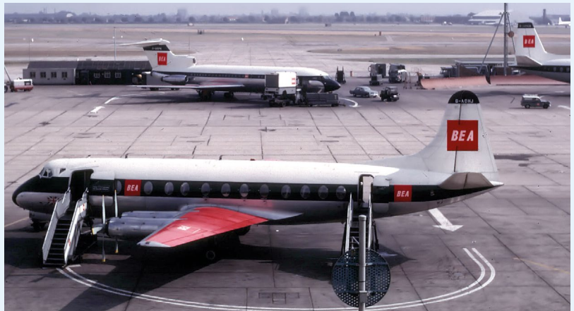
Above: Vickers Viscount 802, G-AOHJ, of BEA at London Heathrow Airport in 1964. Behind is a Hawker Siddeley Trident. The Viscount was a response to the Brabazon Committee's Type IIB design for a short-haul, propeller-turbine powered pressurised airliner. Around 445 Viscounts were built between 1948 and 1963. Adrian Pingstone.
