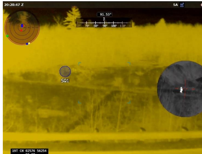
Figure 170: ENVG-B displaying command and control information along with a sight reticle in a picture mode (U.S. Army Photo, 2021)
