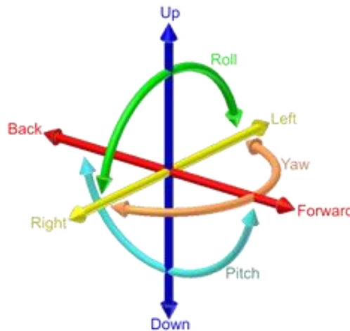
Figure 87: Motion Tracking Sensor degrees of freedom/measurement (Weis, 2018)
