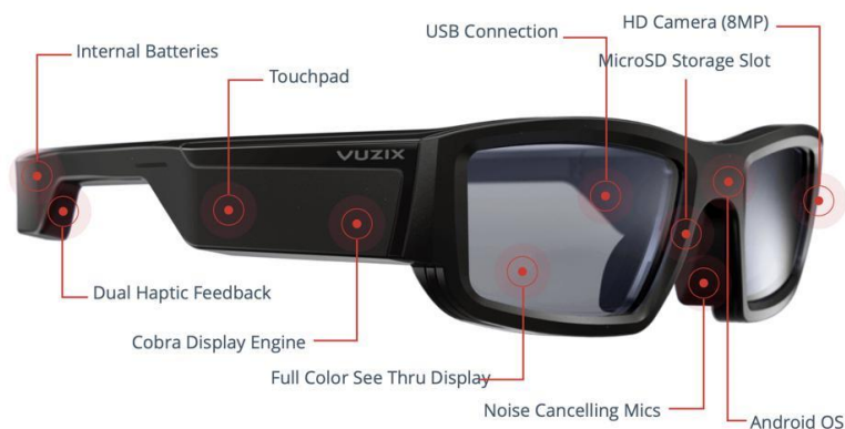
Figure 85: Illustration of sensors on an augmented reality device (Koetsier, 2020)
