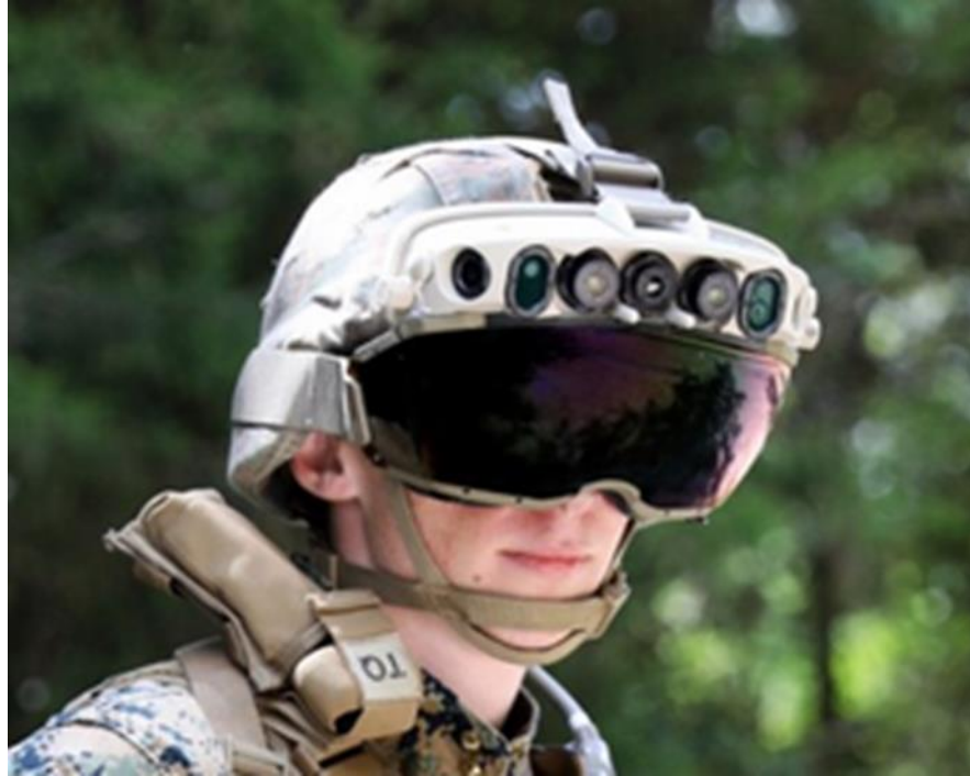
Figure 123: IVAS Cameras and Sensors (PEO Soldier, 2020)
