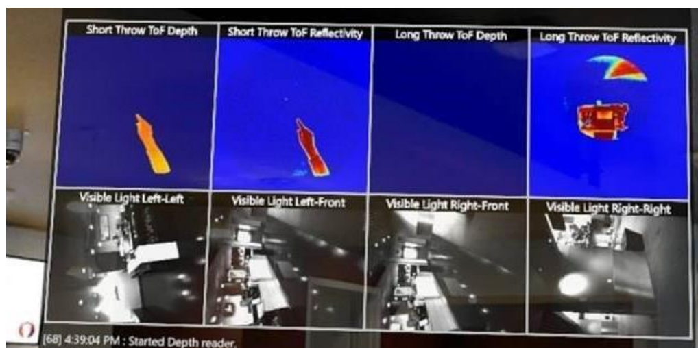
Figure 86: Hololens 2 cameras and resulting images (Davies, 2018)
