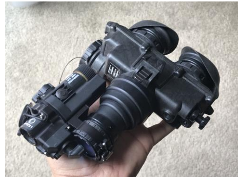
Figure 178: COTI™ Clip-On Thermal Imager attached to an AN/PVS-7 NVG (Image copyright the Firearms Blog, 2019)
