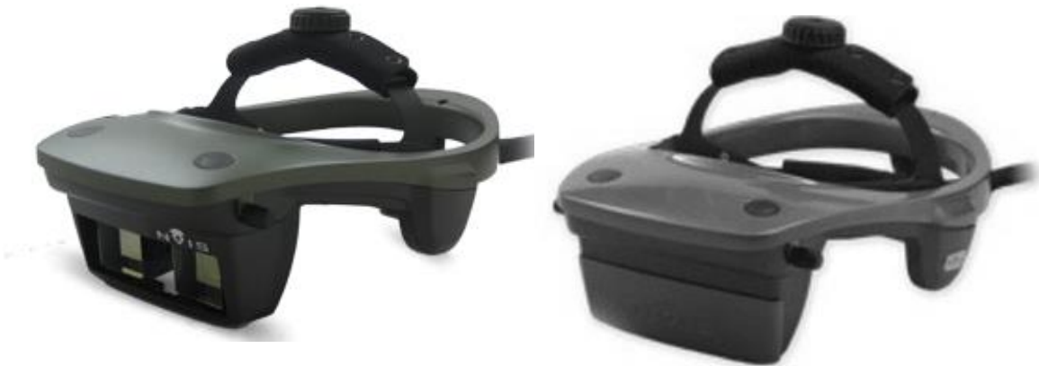
Figure 119: nVisor ST50 showing optical see-through condition (left) and VR condition (right) (NVIS, 2020)
