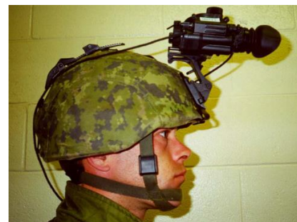
Figure 143: Monocular AN/PVS-14 goggle (in raised position) mounted on a CG 634 Helmet. (Image copyright HSI®)
