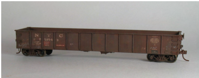
NYC 751943 represents one of 1,000 heavy, all-steel mill gondolas built for NYC in 1929 by Pressed Steel. The cars were numbered 751000-751999 and featured an all-steel body with a wood floor. The model is equipped with Accurail 50-ton ARA trucks, but those will be replaced with the new 70-ton ARA plain-bearing models recently made available by Kadee. John Golden photo.
