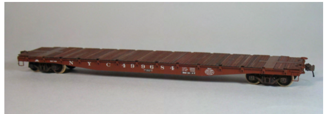
NYC 499684 is a model of a 70-ton 53' 6" AAR flatcar that was derived from a Greenville Car Company design. Central built 1,000 cars at Dispatch Shops beginning in November, 1942, to help handle wartime traffic. This particular lot, 721-F, included cars in the 499300-499599 series. An additional 300 cars were delivered 1943 with 200 going to NYC and 100 going to NYC subsidiary Indiana Harbor Belt and the remainder was delivered in 1950. Photo by Kirsten Golden.
