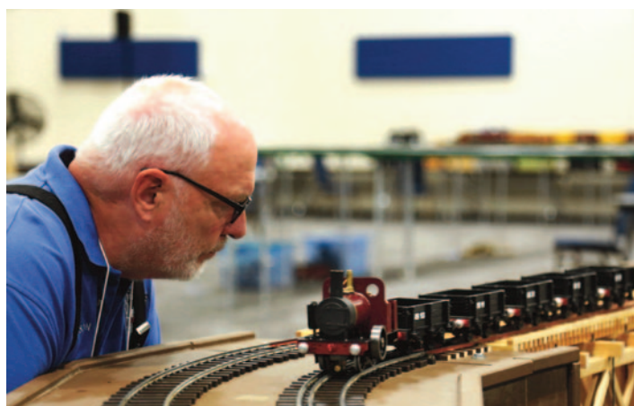
Bob Sorenson of Las Vegas, NV gets up close to his scratchbuilt "Nina". A single vertical cylinder geared locomotive designed by Ernest Glaser and akin to the "Cricket".
