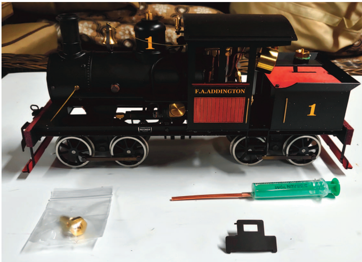
Straight out of the box with the supplied extras. (L-R) Top-off valve, oiling syringe, European style coupler bracket.
