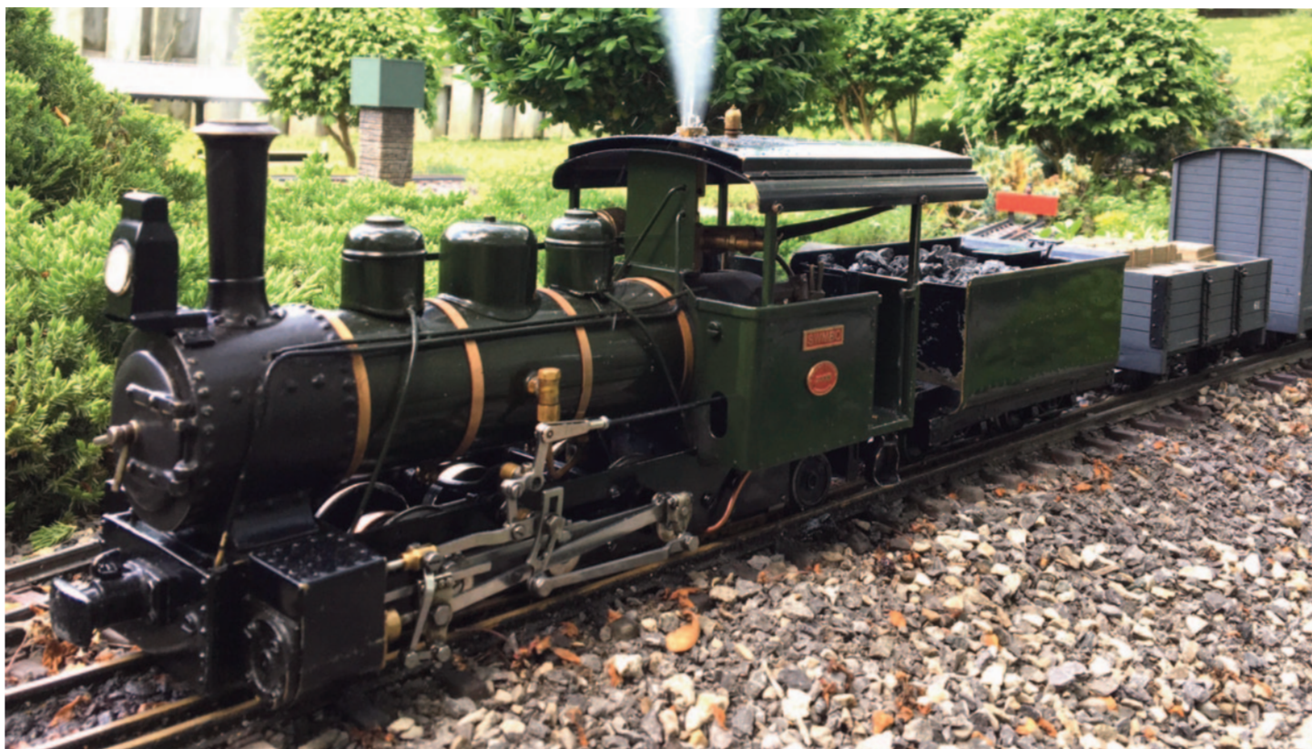
With a good coal fire burning, the safety valve lifts on the author's coal-fired John Shawe Fowler.
