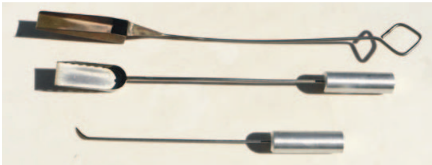
Tools of the coal firing trade: (Top) Two coal shovels — each designed for the specific depth of the firebox and width of the firebox door of a locomotive to ensure even coal distribution and to block excess air from entering while re-coaling. (Bottom) Coal pricker.
