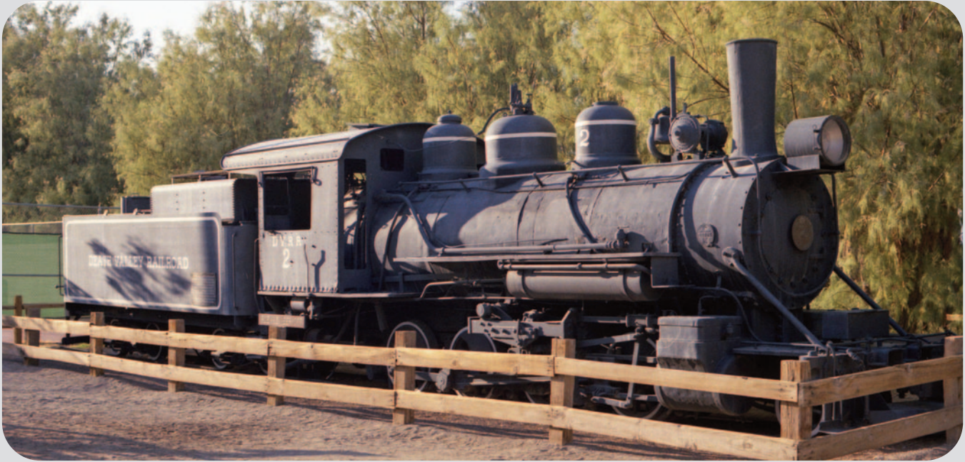
Death Valley Railway 2-8-0 Inside Frame Consolidation in retirement at Furnace Creek, CA.
