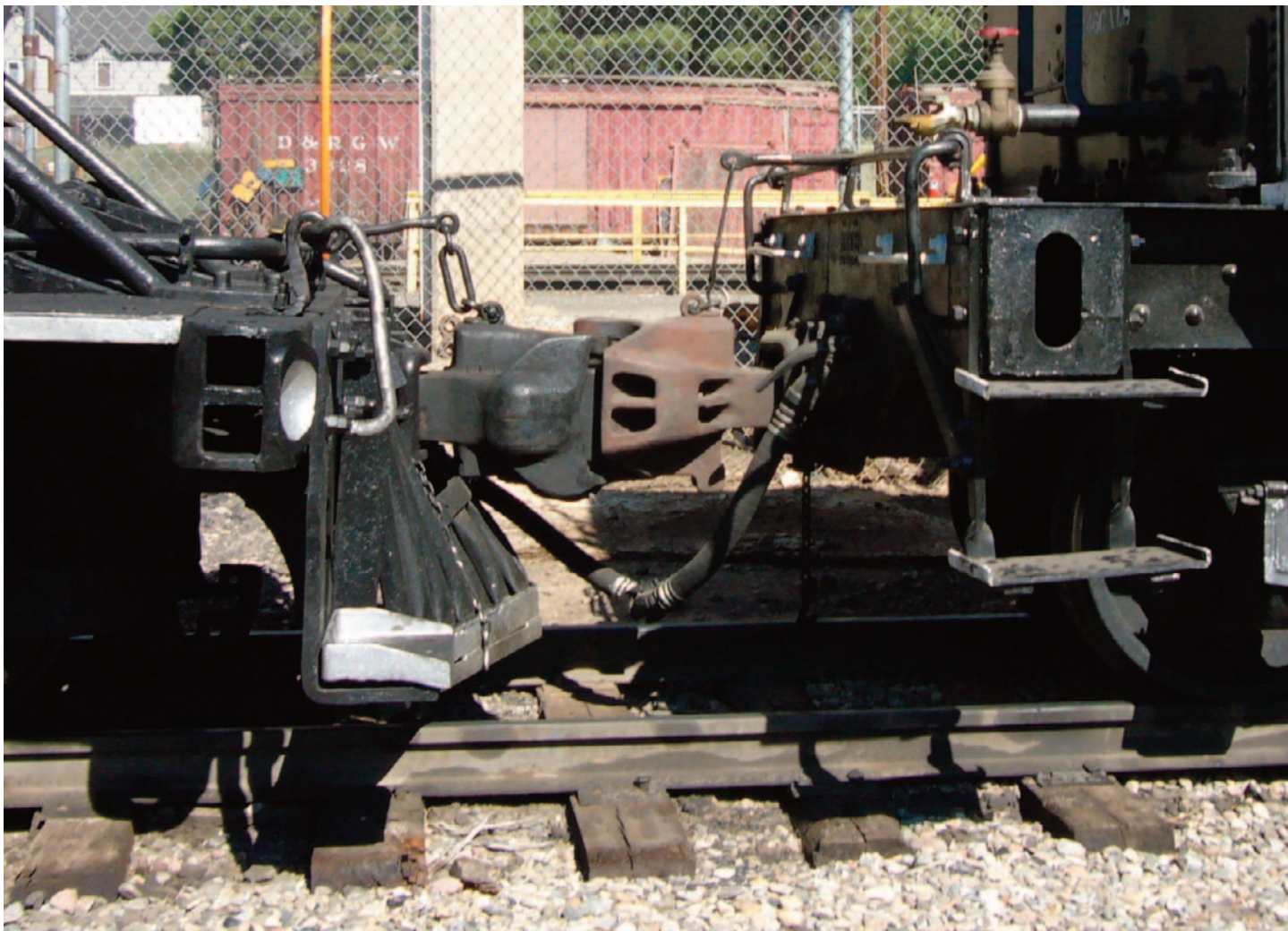
Above: Standard gauge refit of couplers on the D&S RR K-36 (left) and SPng #18 (right)
