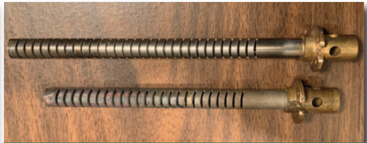
New burner (top) next to old burner for comparison.
