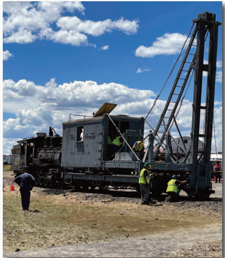
The Friends demonstrated the refurbished D&RGW pile driver which the railroad used in the day to drive posts for trestles. It gets its steam power from the locomotive just behind.
