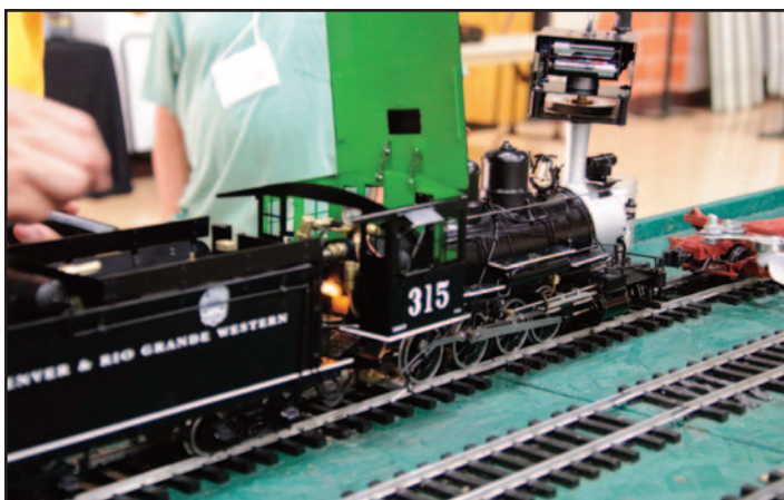
Channing Chen of Accucraft prepares the company's new C-18 for what may have been its first public run. The C-18's ceramic burner glows in the firebox. Like an alcohol burner, this engine has a blower, and will need a fan at startup. **
