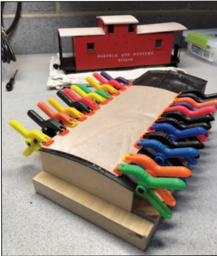
Forming the curve of the roof sections
