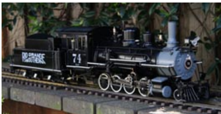
This coal-fired engine is designed and built from the prototype found at the Colorado RR Museum in Golden, CO.
