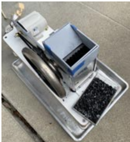
Dennis' scratchbuilt custom coal crusher. This tool can crush larger pieces of coal down to about 1/4-inch.
