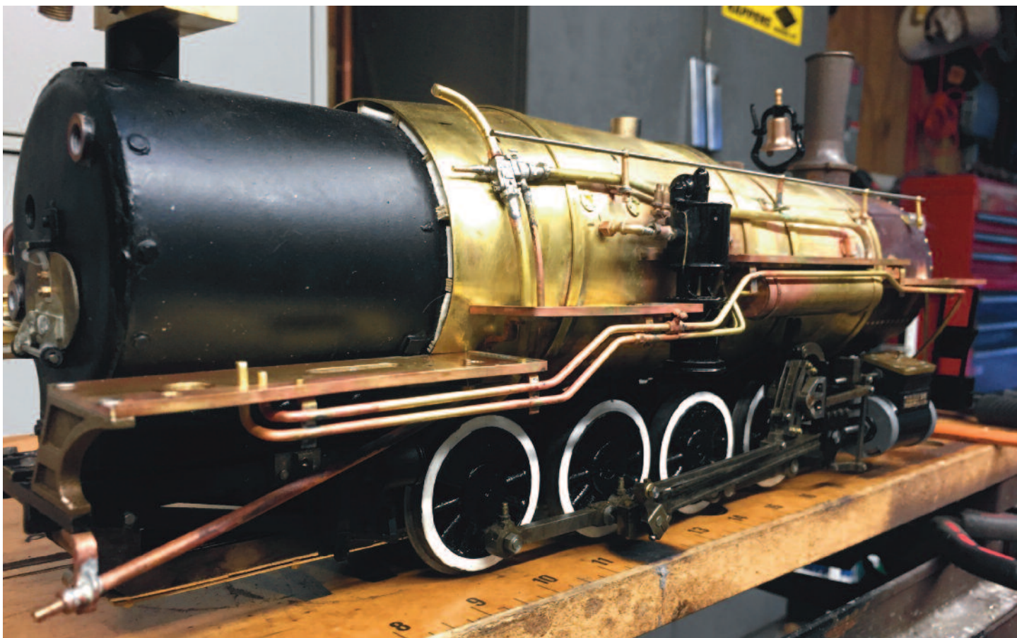
Photo 6 - The right side of the locomotive with the plumbing details in place and the tender water feed line.
