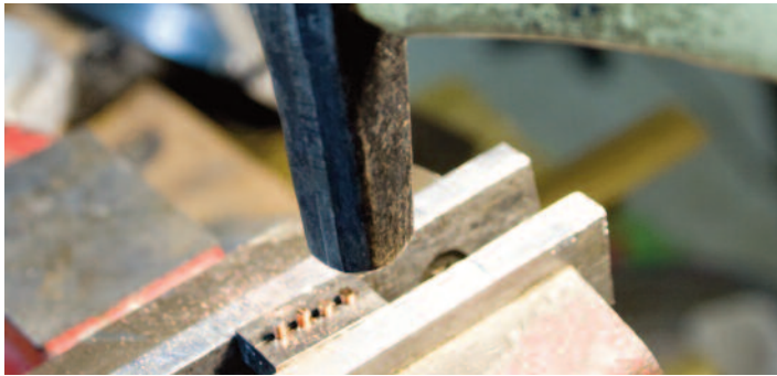
Photo 9 - Rivet heads being formed with a tack hammer.
