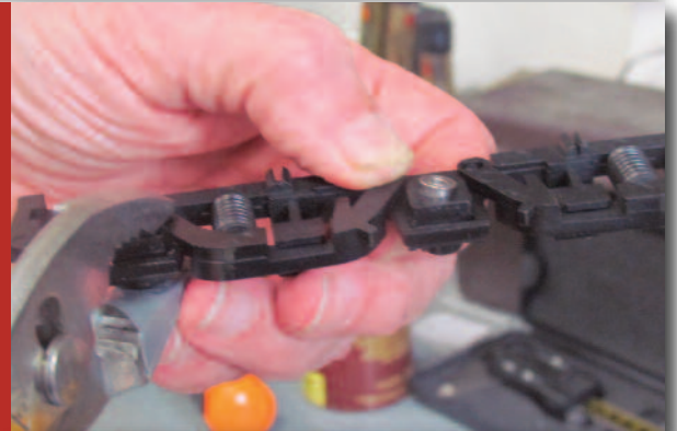
Photo 1 - Pressing the ball bearings into the newly dimensioned journal.
