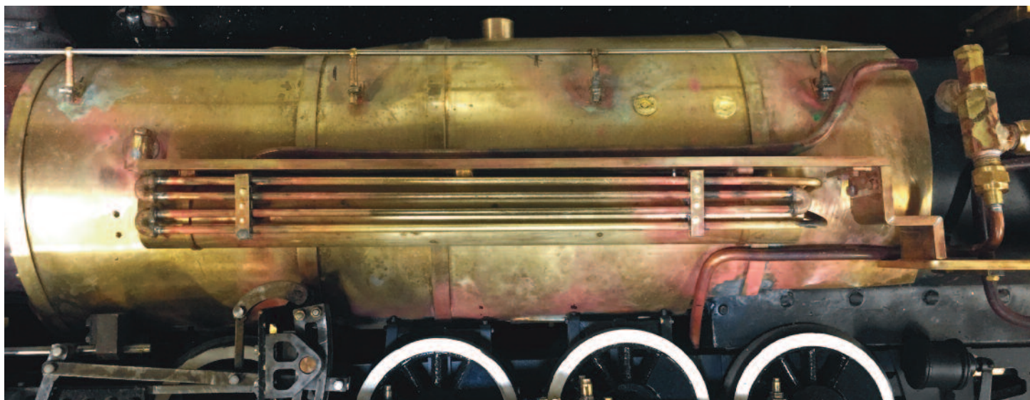
Photo 5 - Check-valve plumbing and steam condenser details
