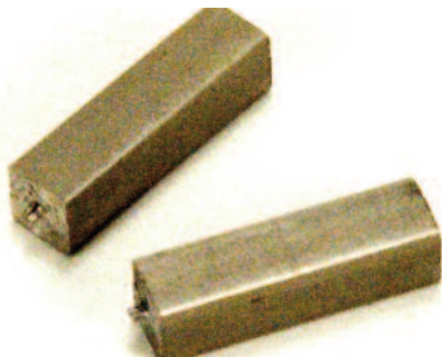
Photo 1 - Two inch-long steel blanks are first cut. Photo 2 - The ends are drilled for 1/16-inch wires.
