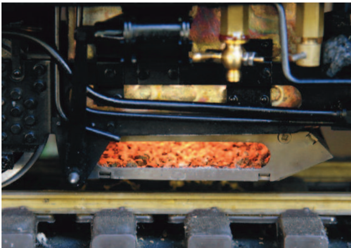
Photo 4 - An impressive glow from the ashpan vents during a coal firing of the locomotive.
