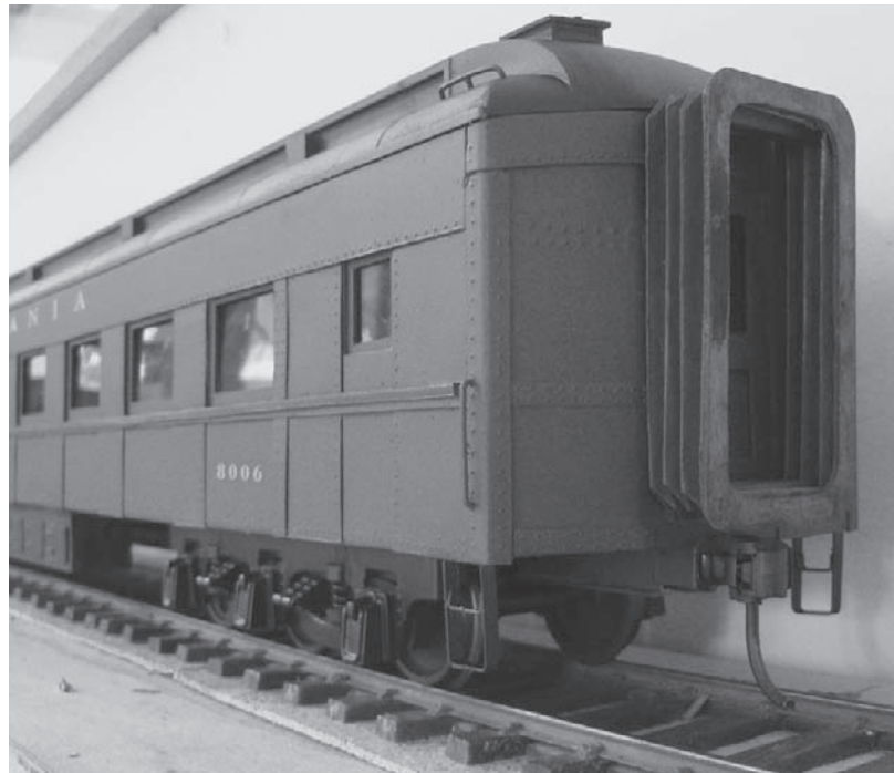
Finished diaphragm: Model of a Pennsylvania Railroad heavyweight with its paper bellows.
