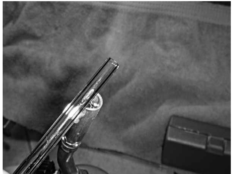
Using a torch to polish the raw end of the glass tube.
