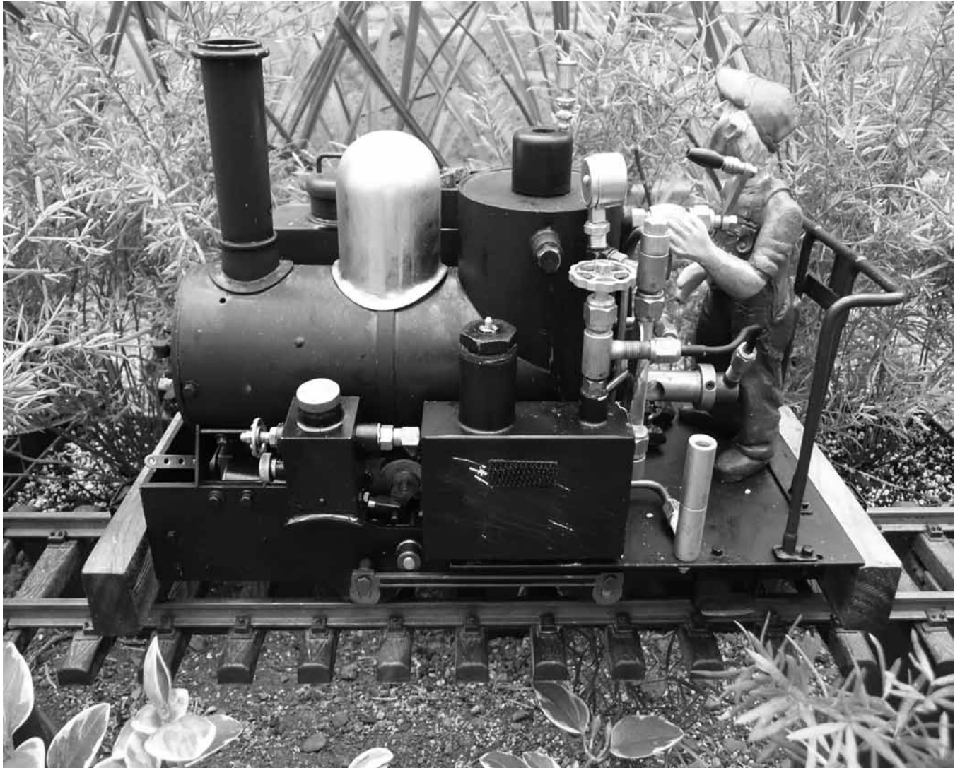
Little Falls No 2 with its port side tank removed shows the relocated butane tank and lubricator and the boiler re-feed system.
