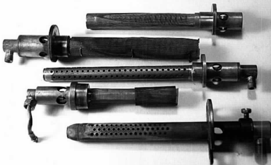
A bevy of burners. From top, stock Ruby burner, modified Accucraft Shay burner (mesh sits above burner where wire is below mesh), Ruby burner with Milton Locomotive Works replacement poker, Cricket burner modified as described in this article, stock Roundhouse Sammie burner.
