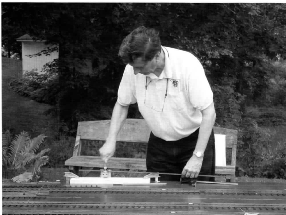
Peter winds a piece of rail through the railbender. Don't try to bend your rail by hand! You will not get a smooth curve that way. The railbender assures smooth, consistent curves.
