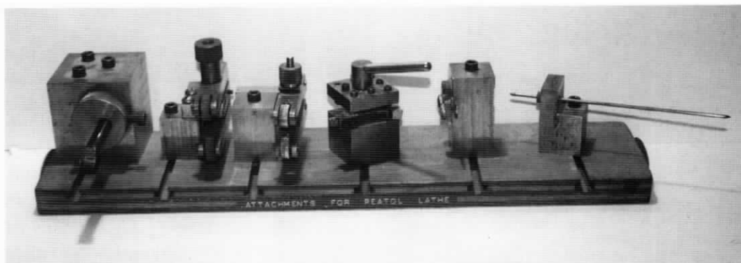
An assortment of tools for the Taig/Peatol Microlathe, all designed and built by the author.
