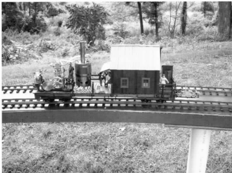
Bob Koenig's "House Car", powered by a Midwest boiler and Graham single cylinder steam motor. The interior of the cabin is fully detailed, and yes, that's a rail bicycle on the rear.
