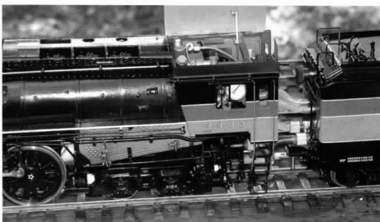
Fireman's side of cab and tender to loco connections for fuel and water.
