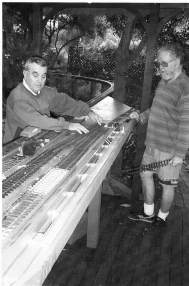
Setting out the position of the track for the sector plate.
