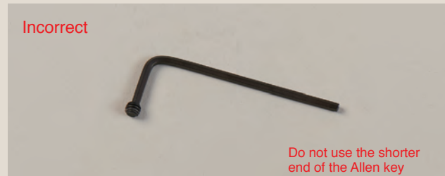
Put the screw on the long axis of the Allen key
