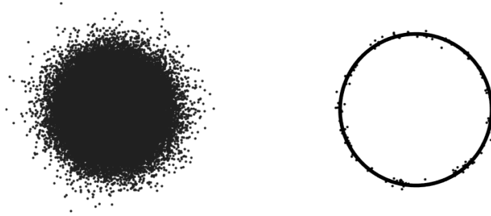
Figure 3.6 A Gaussian point cloud in two dimensions (left) and its intuitive visualization in high dimensions (right). In high dimensions, the standard normal distribution is very close to the uniform distribution on the sphere of radius \sqrt{n} .
