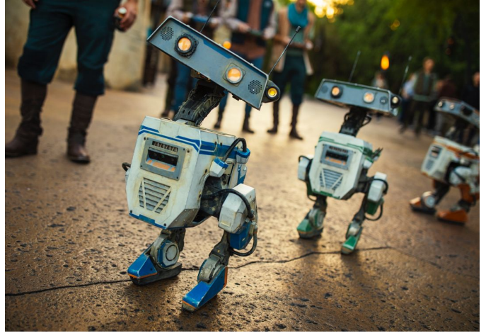
Fig. 1. Three instances of our robotic character performing an unscripted show. Apart from their theming, they are identical. Each robot is remote-controlled by a separate operator.
