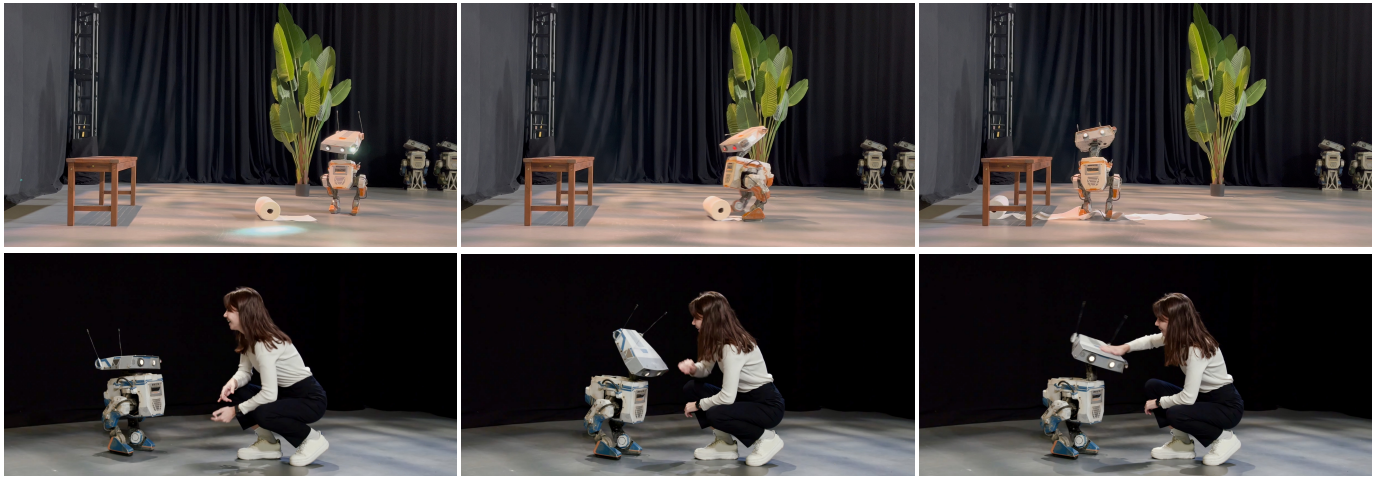
Fig. 10. (Top) The operator uses the proposed puppeteering interface to act out a scene where the robot discovers a paper roll and decides to kick it under the bench. We make use of the head lamp, triggered head animations, and gaze controls to convey initial curiosity. Episodic policies are triggered following the run-up and kick to convey excitement and celebration. (Bottom) The operator puppeteers the robot to interact with a human. The robot is at first shy, then approaches, extends its head, and is rewarded with a head scratch.
