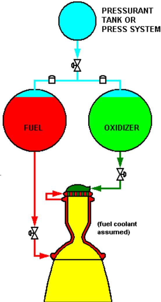
Not really a cycle, since it does not power turbomachinery, but serves as a basis of comparison. While this is the simplest system, it is also the most performance-limited in comparison to pump-fed systems.
