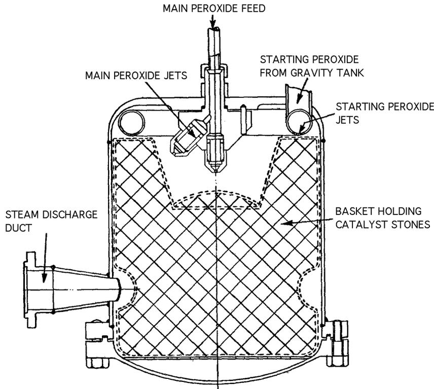
Typical Monopropellant GG Component Layout
