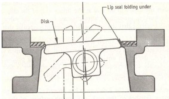
Butterfly valve showing the lip seal and disc rotation
