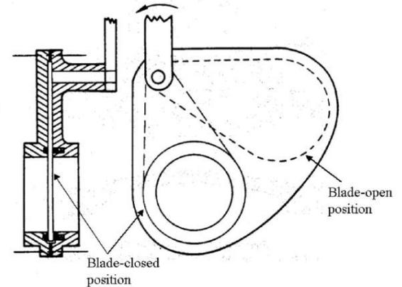
Blade valve - consists of a flat disc that is fixed perpendicular to the flow stream or duct axis.
