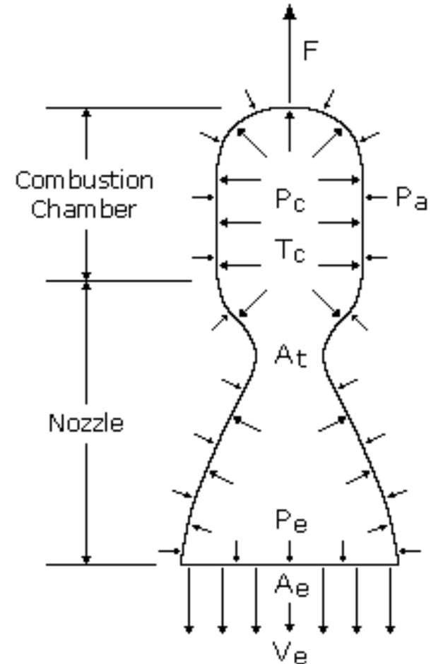
The *total impulse* ( $I_t$ ) is the thrust integrated over the run duration (time,  $t$ )
