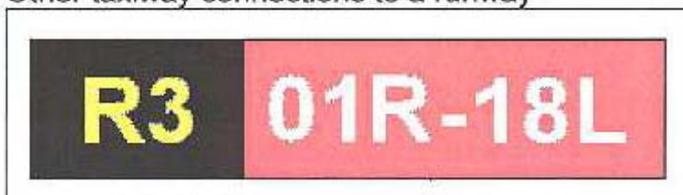
An information sign shall be provided where there is an operational need to identify by a sign a specific location or routing (direction or destination) information. Such a position might be the present "Runway extension " position at the present R5 taxiway. Such a sign shall be a location sign.
