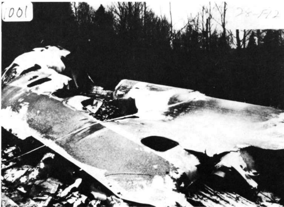
Figure DO4. Fire-damaged fuselage section
