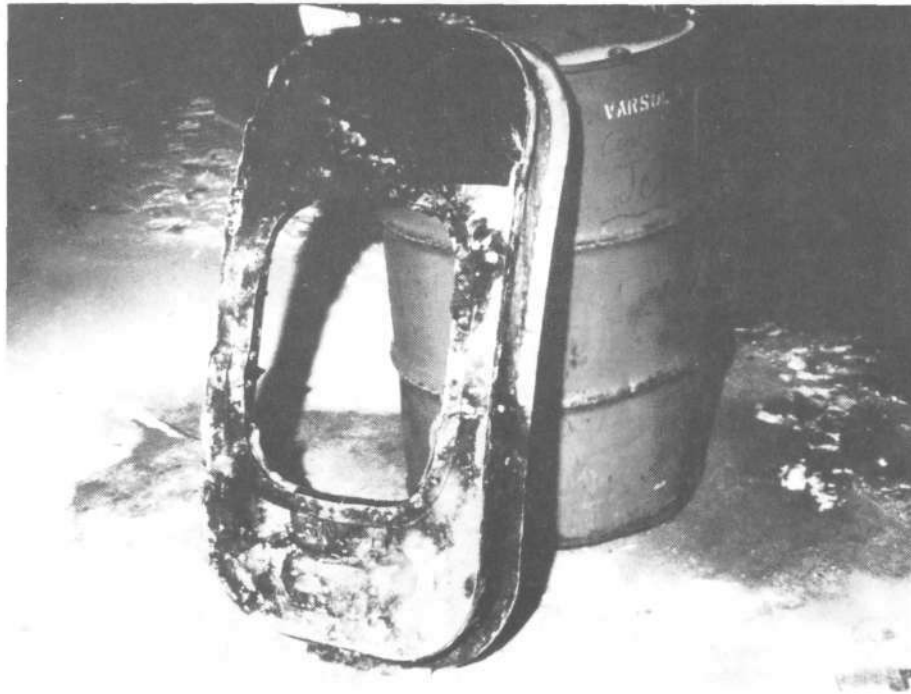
Figure DO5. Emergency exit showing soot deposits around edges
