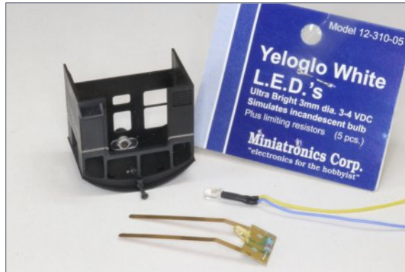
9. The original Kato LED and its Miniatronics Yelogle White replacement for the rear headlight in the cab.
