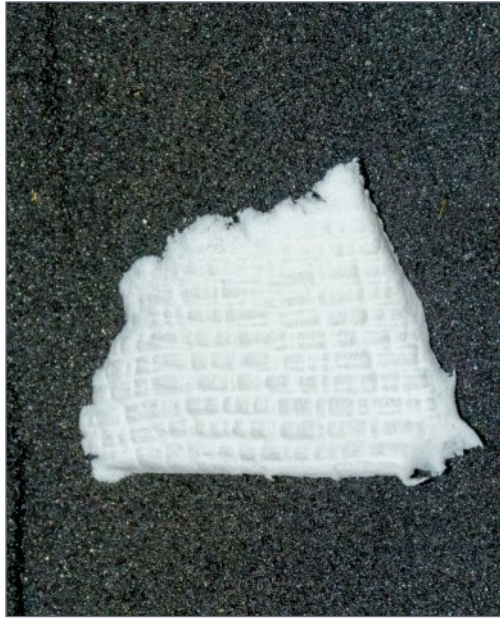
5. Set pavement pavers indented horizontally across the clay.
