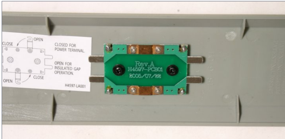
11. The E-Z Track 9" terminal rerailer can be used either as power-connector or to provide an electrical insulation gap.
