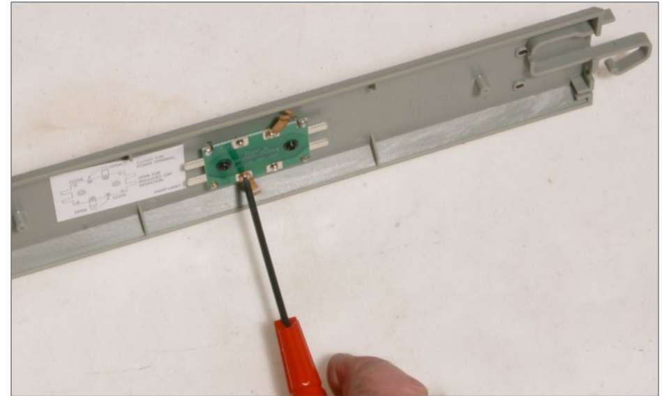
12. Loosen the screws, and the pair of pivoting copper contacts can be rotated 90 degrees to disconnect the two halves of the rails to allow the rerailer to serve as an electric block. There are power connections on both sides of the pivoting contacts, so power for the two blocks can be connected to both blocks at this one site.
