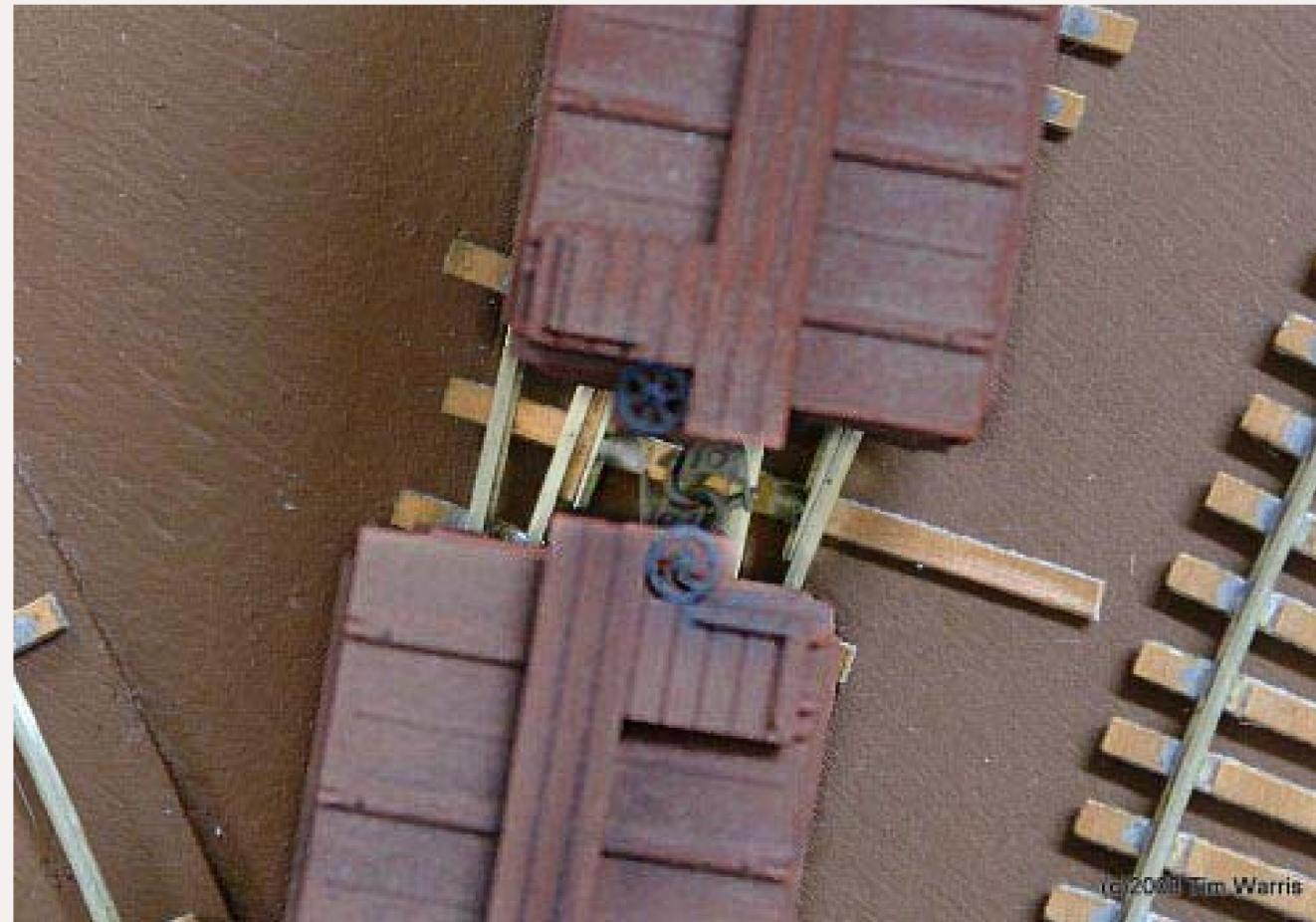
**FIGURE 1:** The thing to watch with S curves is coupler alignment – which actually doesn't look too bad in the above photo. In this issue, our trackwork columnist takes another look at that trackwork bug-a-boo, the S curve.
