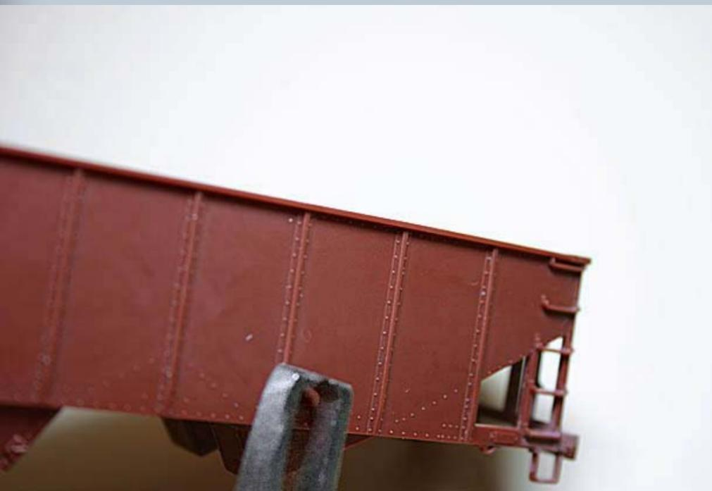
securing the styrene I place with styrene cement.
