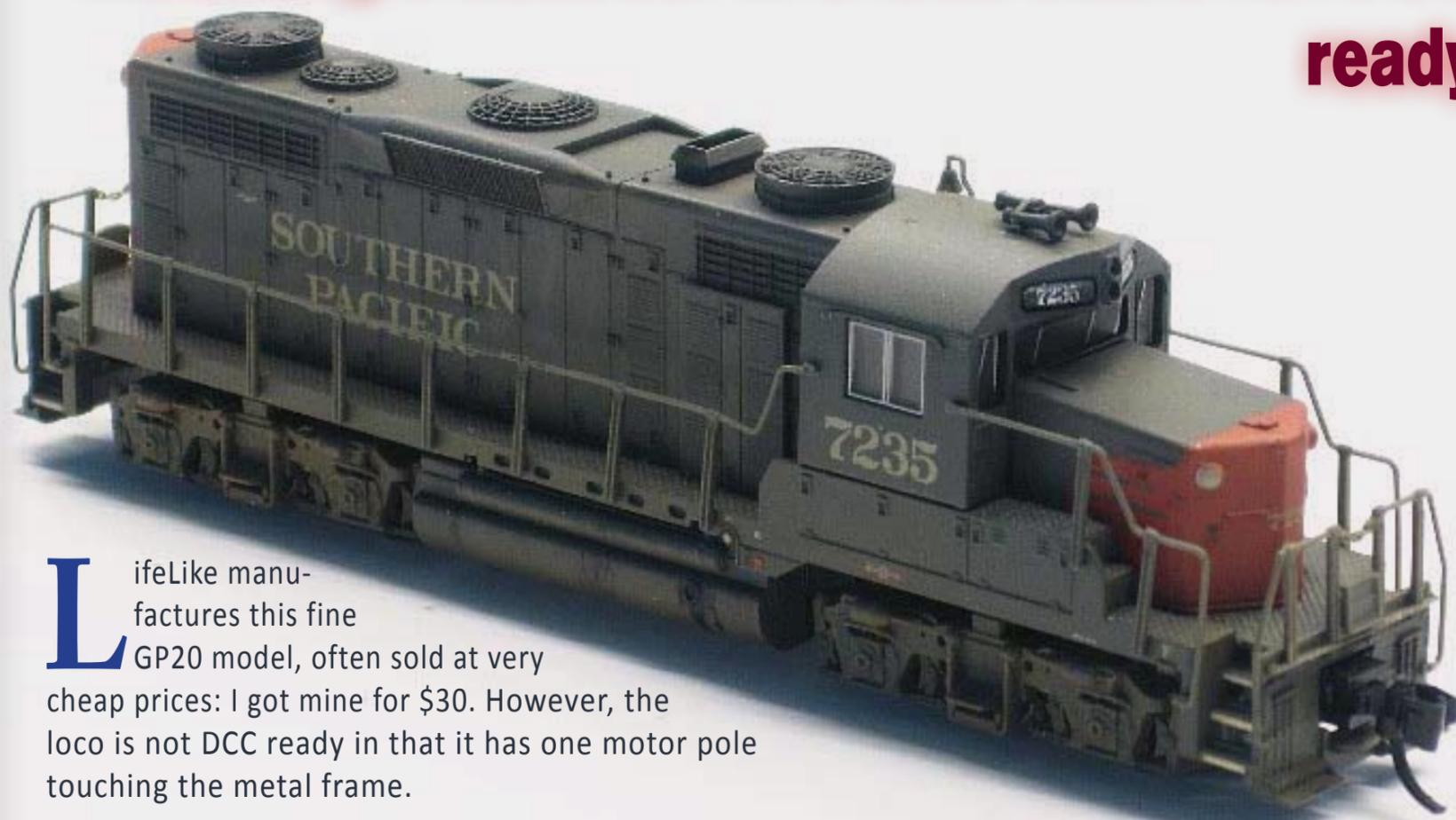
**L**ifeLike manufactures this fine GP20 model, often sold at very cheap prices: I got mine for \$30. However, the loco is not DCC ready in that it has one motor pole touching the metal frame.
