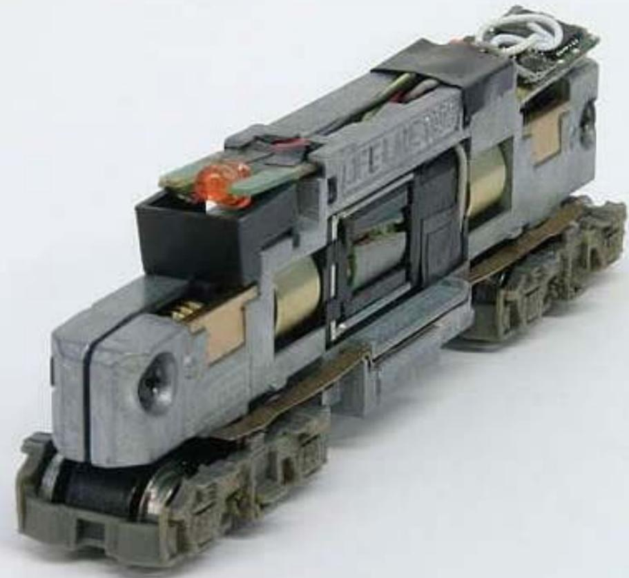
**STEP 8:** I then put some tape to firmly hold the wires in place and put the shell and tank back on.
