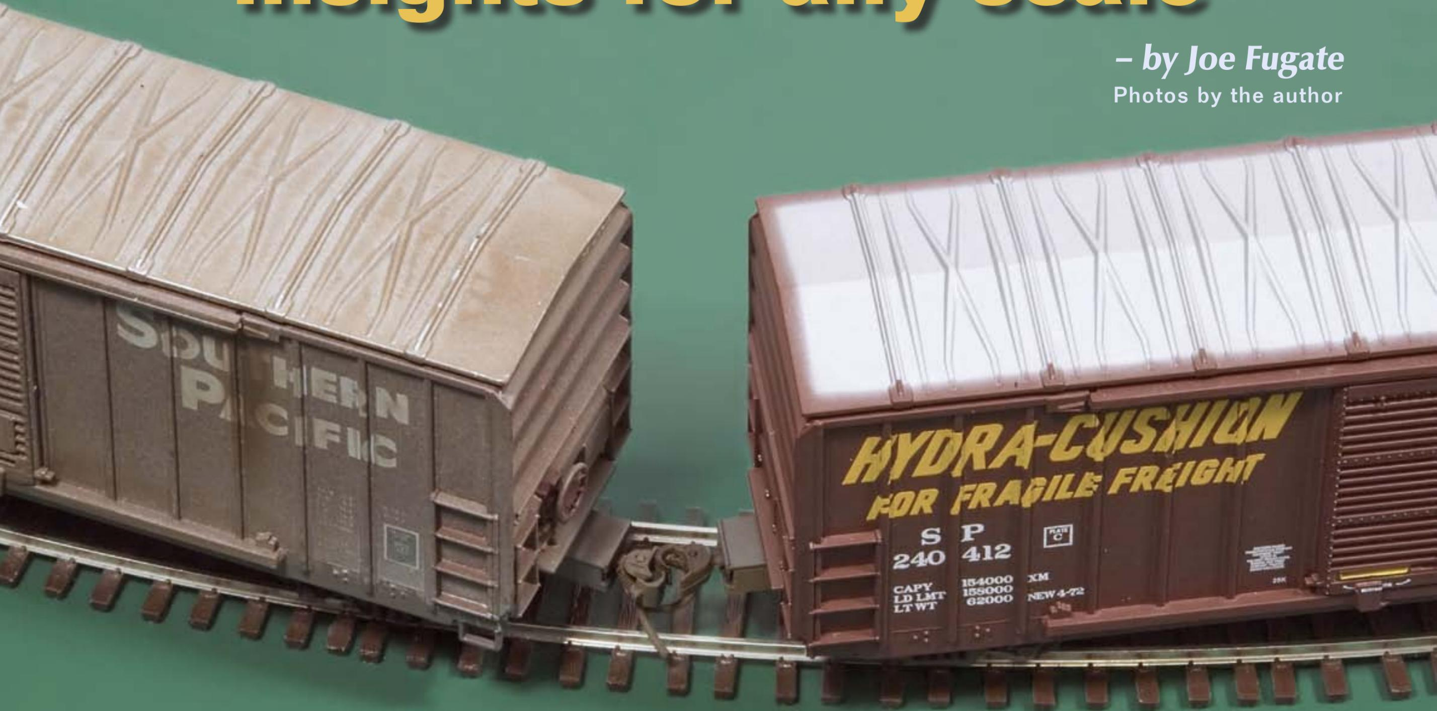
FIGURE 1: Here's one of the big problems a with a curve that's too sharp - poor coupler alignment. These cars can't couple automatically since the jaws don't engage. This article presents some new curve radius insights that came out of a discussion on the Layout
