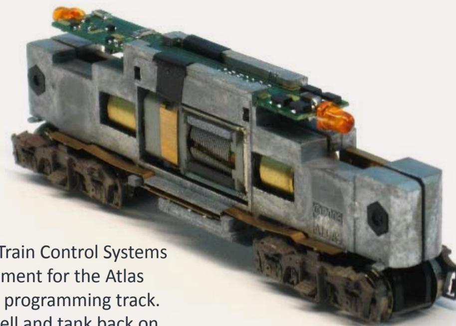
**STEP3:** I replaced the PC board with an Train Control Systems ASD4 drop in decoder: a perfect replacement for the Atlas board! Next I tested the decoder on the programming track. Everything went smooth, so I put the shell and tank back on and I was ready to fine tune CVs and run my Geep!
