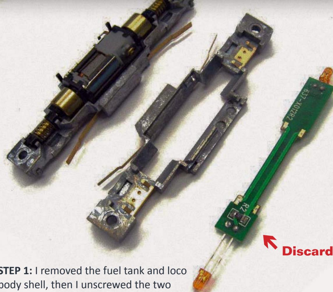
**STEP 1:** I removed the fuel tank and loco body shell, then I unscrewed the two ends of the frame weight and set them apart. This allowed me to remove the original PC board and discard it.
