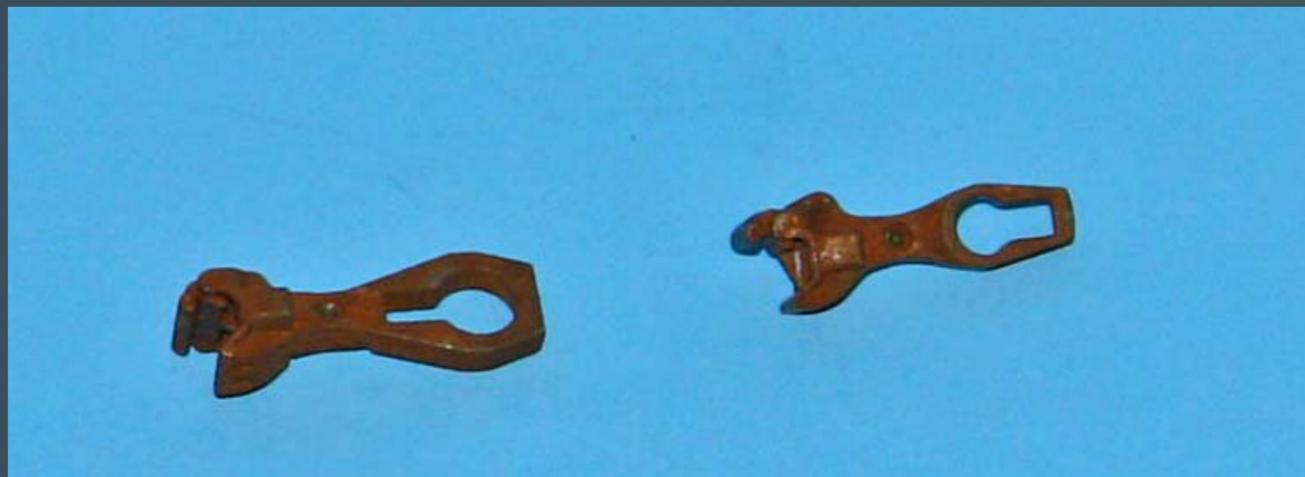
Figure 1: EC87 (left) and EN87 Couplers.
