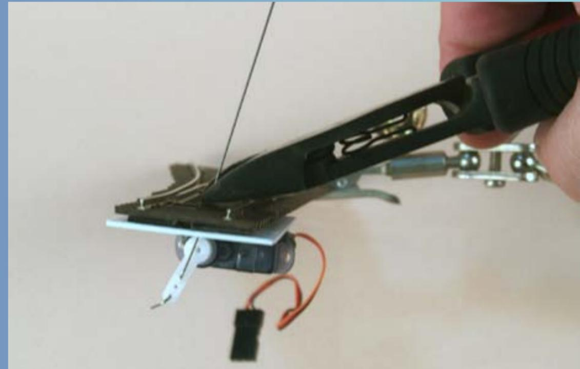
Before cutting off the excess wire, gently move the servo arm to one side as this pulls the wire down in to the hole. If you cut it off too close then when you move the arm to the side, the wire may pull out of the hole.
