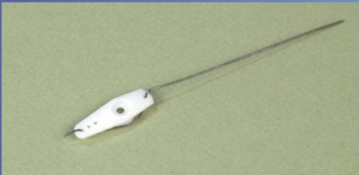
Bend the 2 ends down like this. The wire will now stay on and it won't interfere with the mounting hole. Note that there are little set screw-based devices made for attaching wire to servos but these are normally best avoided. The screws will work themselves loose over time and disaster will follow.
