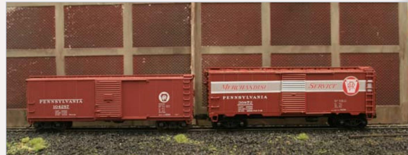
**FIGURE 4: Atlas rebuilt X26C and IM X29B in one of the colorful "Merchandise Service" schemes illustrate the transition-era variety in boxcar height.**
