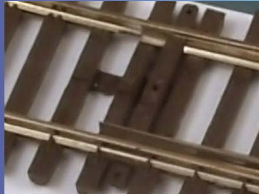
The micro-engineering turnout has a small hole in the middle of the throw-bar that will be used for the actuating wire. If there isn't a hole in your turnout then drill one with a small drill a little larger than the wire.
