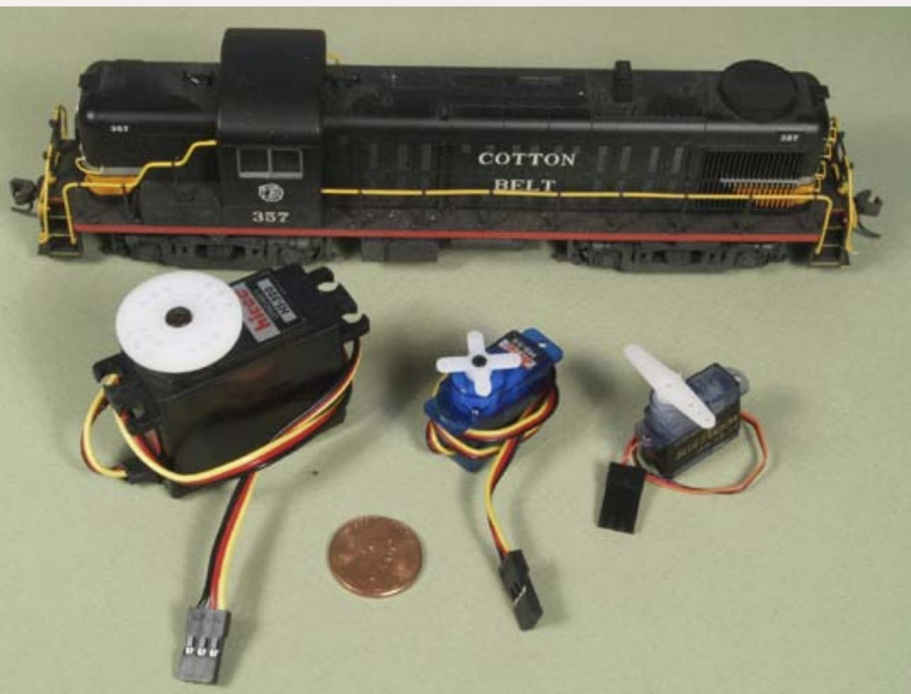
**FIGURE 1: Three sizes of R/C servos with an HO scale locomotive and a penny for size comparison. From the left are a standard, mini and micro servo. All 3 servos have a standard 3-pole plug and despite their different sizes and all respond identically to standard R/C servo signals. The white servo arms can be replaced by a wide variety of different size and shapes for connecting to different devices. In this article I show a few uses for model railroads including turnouts and semaphores.**
