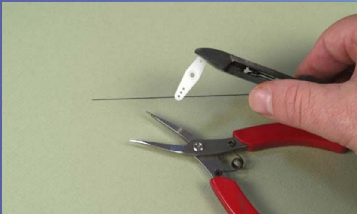
One end of the servo arm is shortened by cutting it off with diagonal pliers to give it sufficient clearance. Be certain not to cut the last hole.
