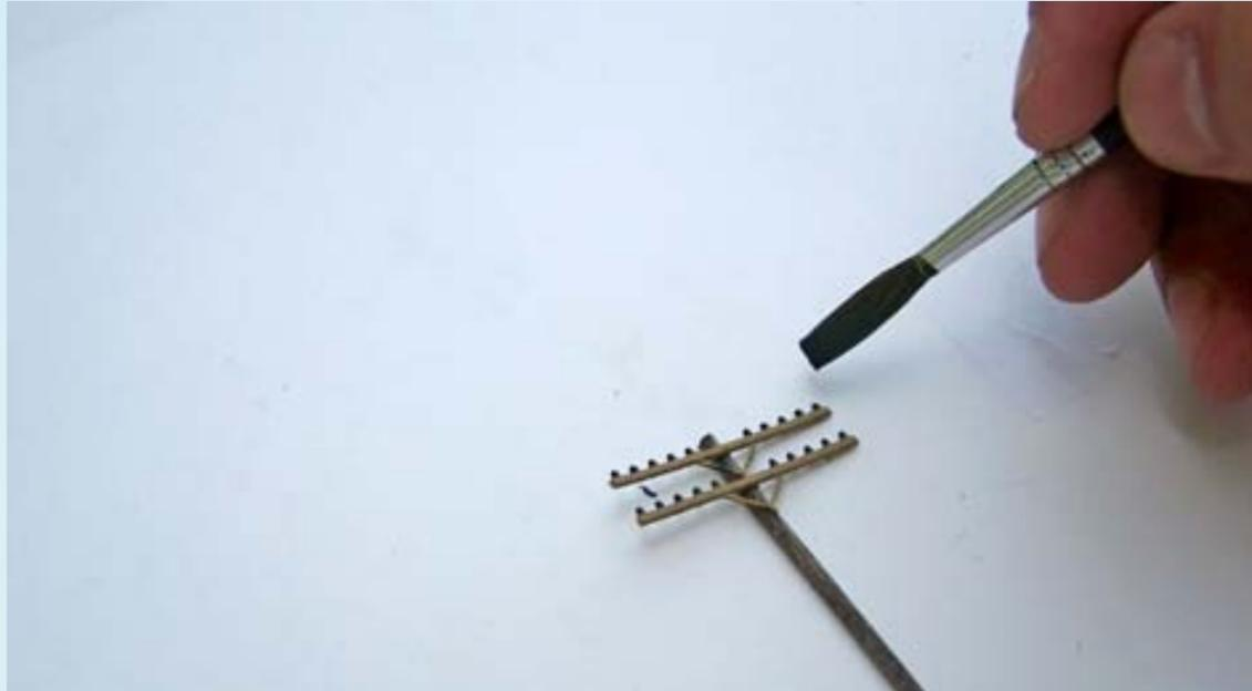
Figure 10: Paint the insulators.
